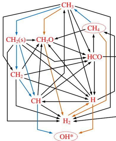
Figure 1. The production pathway of OH\* chemiluminescence.
