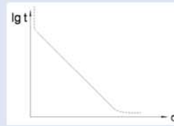
General relation between life time t and load \sigma for brittle solids
