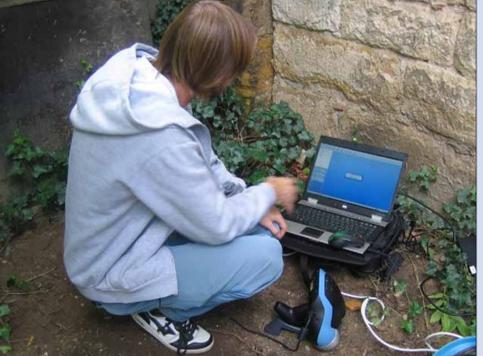
Generation of a 3D-surface by means of a handheld laser scanner and the software Geomagic®
