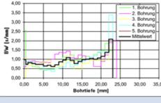
microdrilling resistance measurement: Lowest hardness is observed near to the surface up to a depth of about 6 mm. After this zone the hardness profile tends to increase until the sound material is reached in about 23 mm depth.
