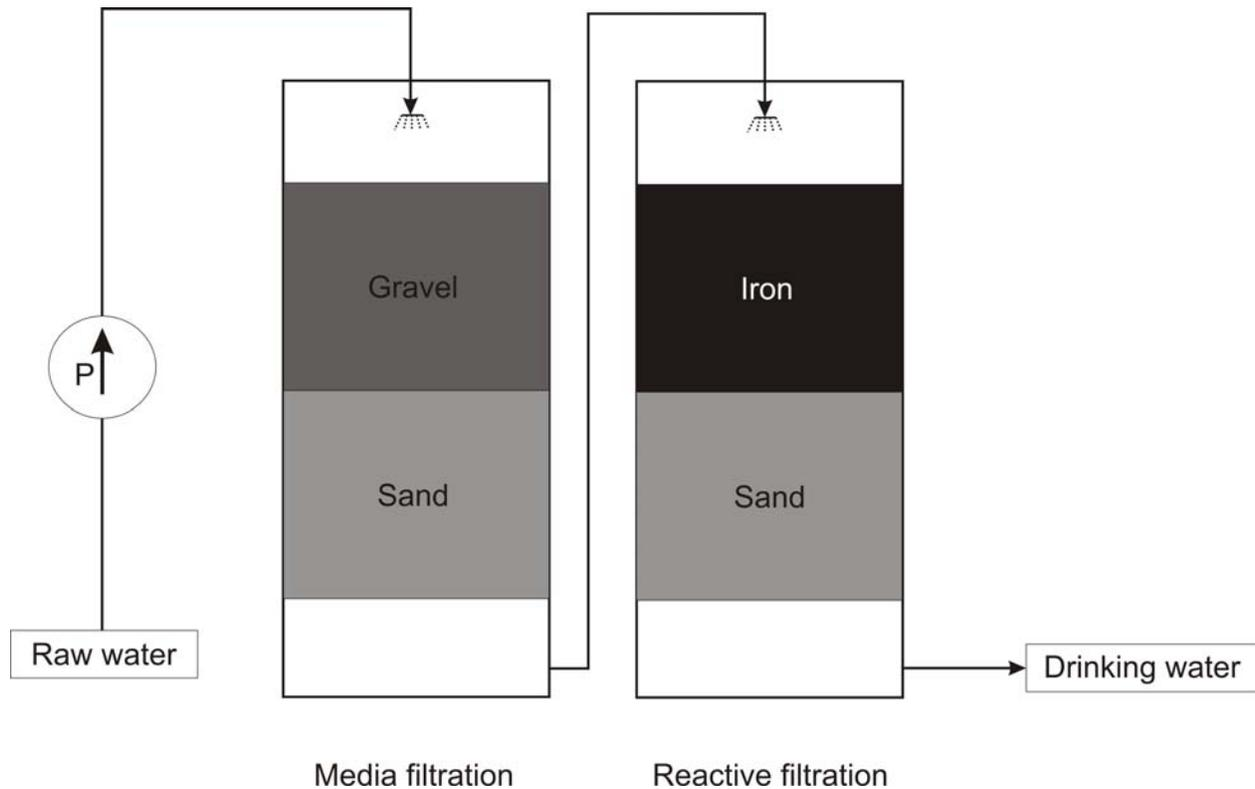
**Figure 1:** Flow scheme of treatment concept. Potential materials are enumerated without care on their relative proportions. In the reactive filtration bed, sand and iron particles are mixed. The volumetric proportion of Fe<sup>0</sup> should not exceed 50%.
