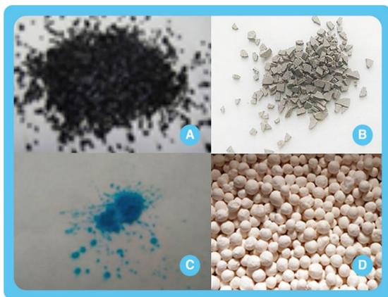
Fig.2 Adsorbents proposed in the VSA/VPSA adsorption technology: a) activated carbon, b) MIL-53(Al) metal-organic framework, c) CuBTC metal-organic framework, d) zeolite 13X.
