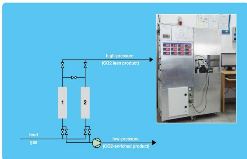
Fig.3 Schematic diagram and a view of the VPSA installation
