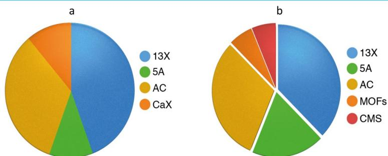
Fig.1 Solid adsorbents used in VSA/VPSA units: a) pilot CO<sub>2</sub> capture units, b) laboratory CO<sub>2</sub> capture units
