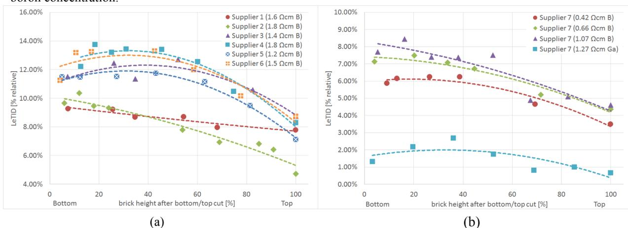
**Fig. 1.** Dependence of relative efficiency degradation after LeTID treatment (75°C, 1 sun, 24h) on relative brick height (after bottom / top cut) for (a) HPM wafers from different wafer suppliers (“1” to “6”) and (b) standard mc-Si wafers from another supplier “7” with different boron doping levels and gallium doping.
