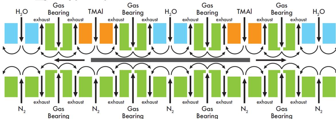
**Figure 1:** Sketch of in-line spatial ALD concept [6]. The TMAI and  $\text{H}_2\text{O}$  half-reaction zones are separated by  $\text{N}_2$  curtains. Contactless transport of the wafer is facilitated by  $\text{N}_2$  gas bearings below the wafer.
