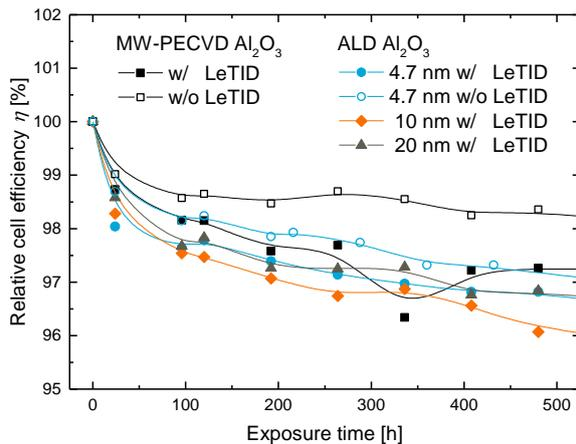
**Figure 5:** Relative cell efficiency degradation for MW-PECVD and ALD  $\text{Al}_2\text{O}_3$  passivated mc-Si PERC cells with susceptible (w/ LeTID) and LeTID controlled (w/o LeTID) process sequence.
