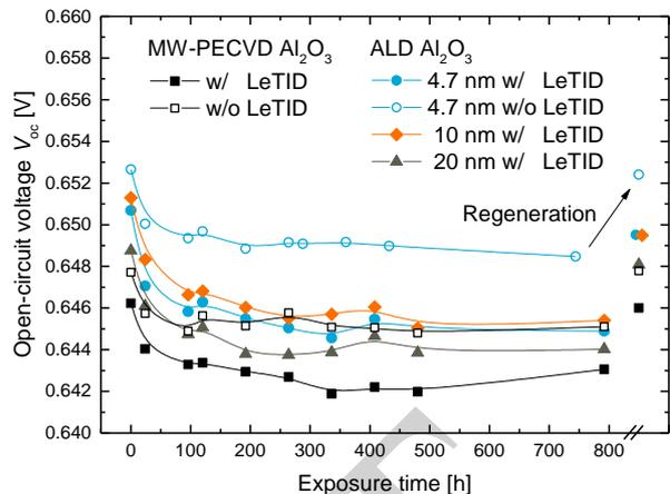
**Figure 6:** Real open-circuit voltage measurement during degradation for MW-PECVD and ALD  $\text{Al}_2\text{O}_3$  passivated mc-Si PERC cells with susceptible (w/ LeTID) and LeTID controlled (w/o LeTID) process sequence.
