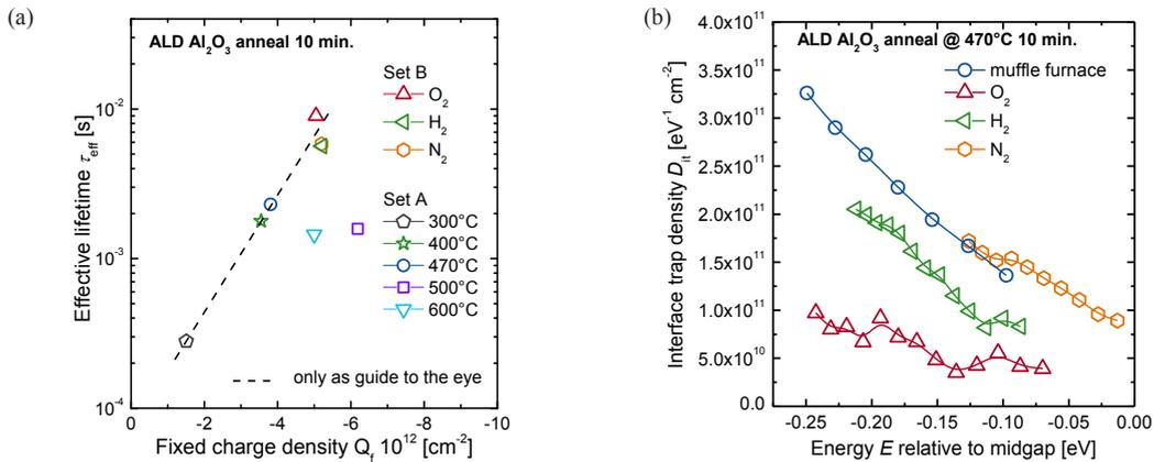
Fig. 2. (a) Maximum  $\tau_{\text{eff}}$ -values as function of the fixed charge density  $Q_f$  and (b) interface trap density  $D_{\text{it}}$  as function of the energy  $E$  relative to the midgap energy  $E$ .
