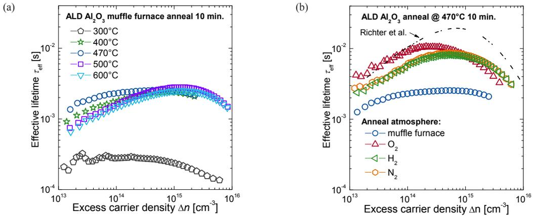
Fig. 1. Injection dependent minority carrier lifetime  $\tau_{\text{eff}}(\Delta n)$  of 30 nm thick ALD  $\text{Al}_2\text{O}_3$  films
