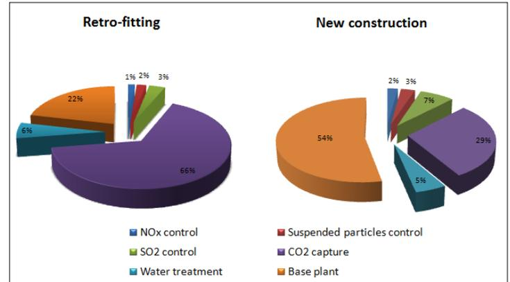
Figure 1.2: Structure of CO<sub>2</sub> capture costs for retro-fitting and new construction
