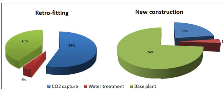
Figure 1.5: Structure of CO<sub>2</sub> capture costs for retro-fitting and new construction
