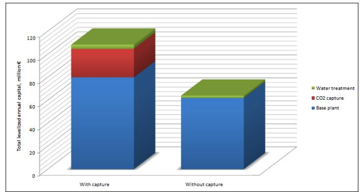
Figure 1.6: Comparison of construction costs for gas plants with and without CCS
