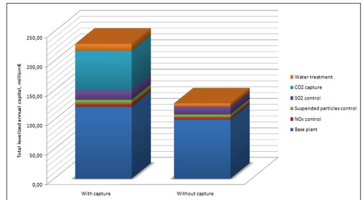
Figure 1.3: Comparison of construction costs for coal plants with and without CCS
