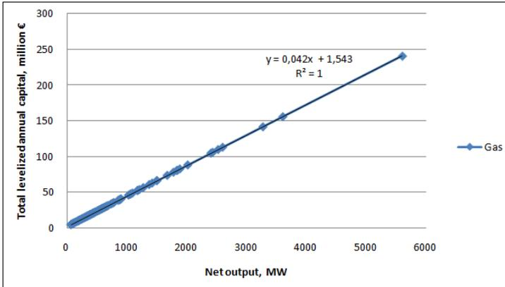
Figure 1.4: Relationship between total levelized annual capital and net output of the gas power plant
