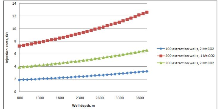
Figure 3.1: Dependence of injection costs on well depth, well number and CO<sub>2</sub> injection rate
