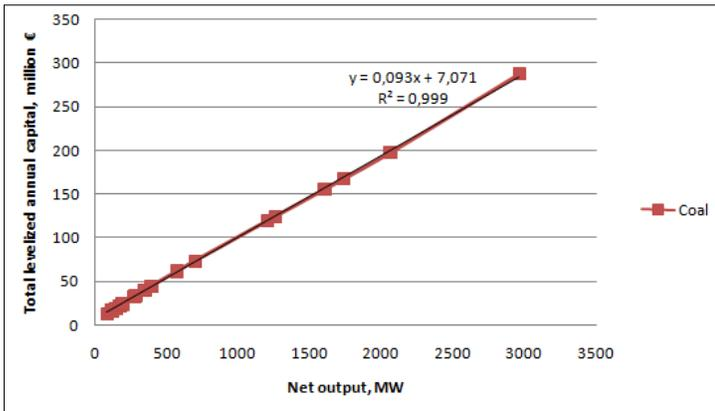
Figure 1.1: Relationship between total levelized annual capital and net output of the coal power plant
