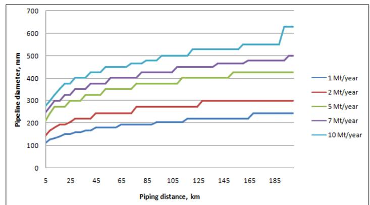
Figure 2.1: Relationship between transportation distance, annual CO<sub>2</sub> flow and pipeline diameter
