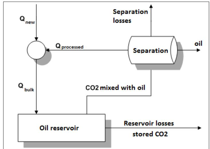
Figure 3.3: Concept chart of CO<sub>2</sub> and oil flows during EOR operations
