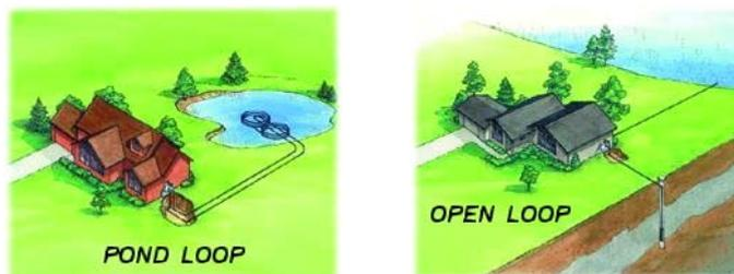
Figure 4. Scheme of a pond (lake) loop and an open loop design. Source: PA Hydronic Company.
