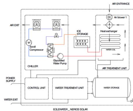
Fig. 2.1: Schematic representation of the process
