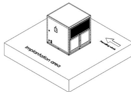
Fig. 3.1: Suggested orientation of the machine
