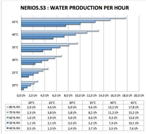
Fig. 2.3: Eole's Water production estimates according to climate conditions
