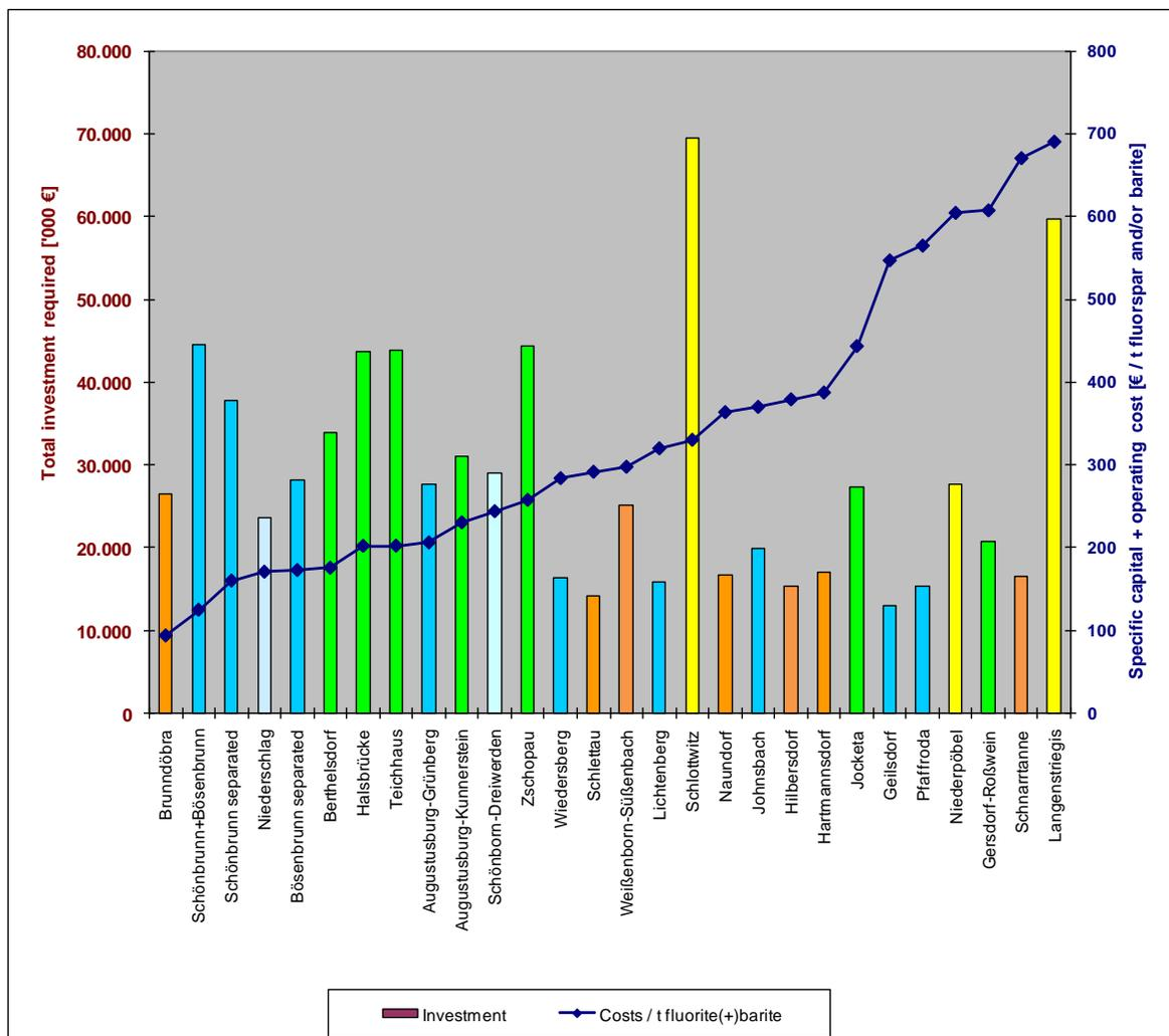
Figure 9: Fluorspar and barite deposits and occurrences sorted after specific costs [statical costs, €/t barite or fluorite] (line). Columns mark the investments necessary to prepare and develop the mine and to construct a processing plant
