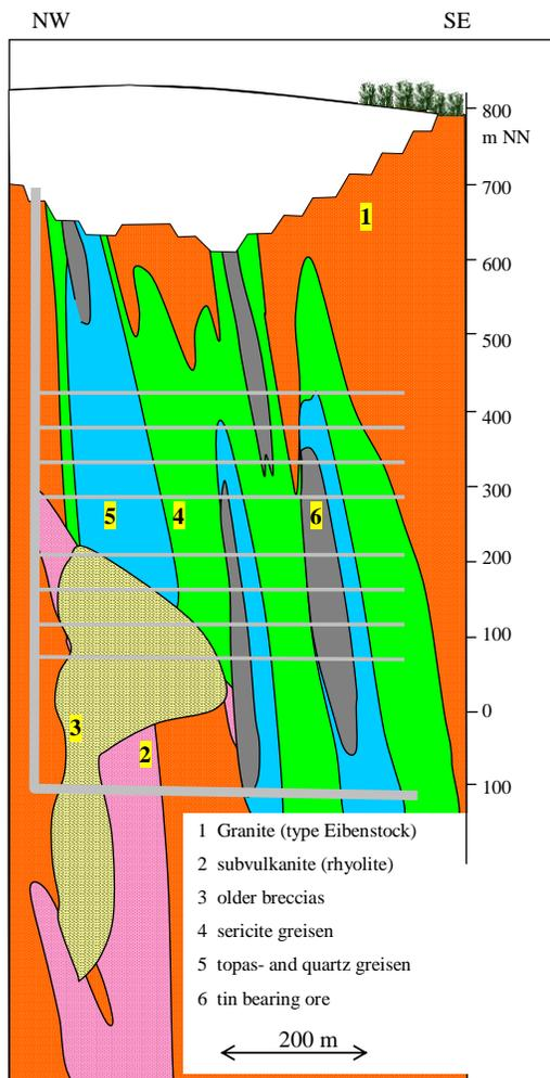
Figure 8: Section of the central part of the Gottesberg tin deposit and proposed extraction by open pit and sublevel stoping according to option 2
