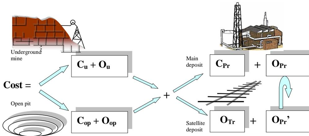
Figure 6: Calculation scheme applied for the determination of direct costs of the potential mines. Capital letters: C = capital costs, O = operating costs; indices: <sub>u</sub> = underground; <sub>op</sub> = open pit; <sub>pr</sub> = processing; <sub>tr</sub> = transport
