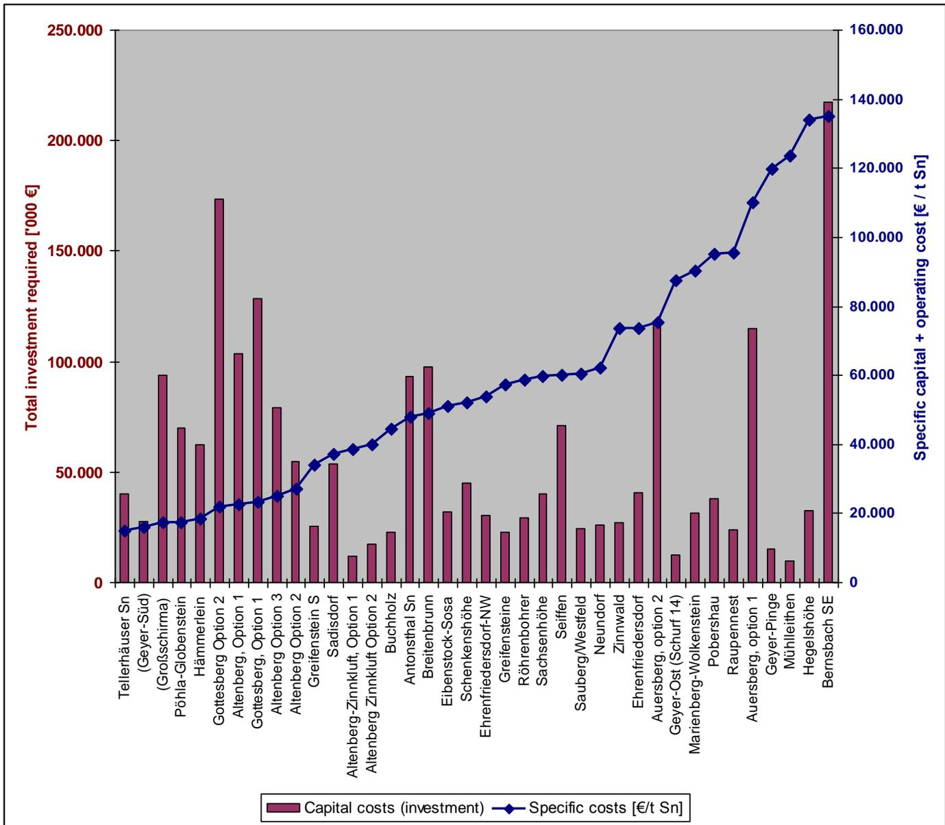
Figure 7: Tin bearing deposits and occurrences sorted after specific costs [fin.-math. average costs, €/t Sn in concentrate] (line). Columns mark the investments necessary to prepare and develop the mine and construct the processing plant. The costs of objects shared between several occurrences are assigned to them in proportion to their production rate
