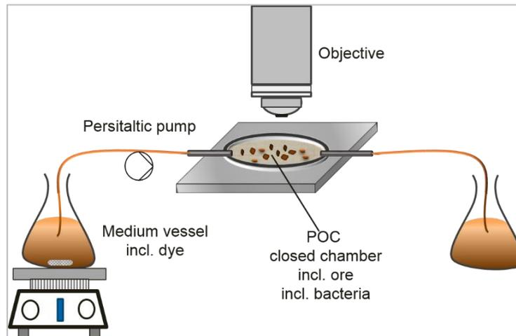
**Fig. 2:** Schematic drawing of an experimental flow chamber set-up for *in-vivo* observation of biofilm formation on minerals. Minerals can be fixed within the chamber in either as grains or as thick sections.
