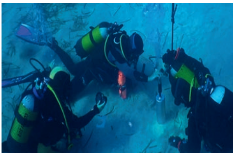
Extraction of cores to analyse solid rocks, picture: Scientific Diving Center, 2011
