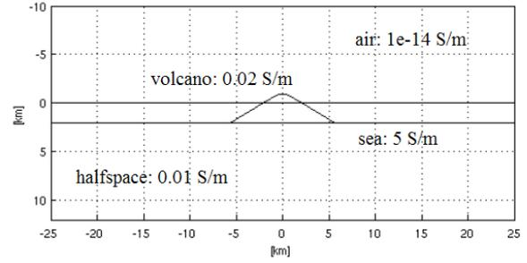
**Figure 2:** Section of the 2D model including the electrical conductivity distribution.
