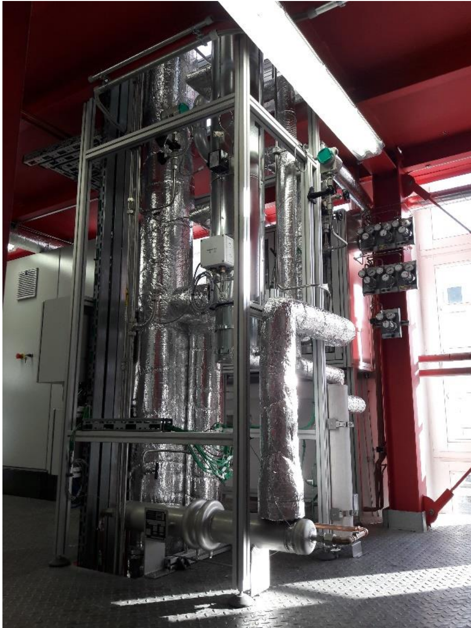
Methanol-to-olefins part of the test plant
