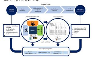
The project aims to support ergonomists and engineers in appropriately evaluating, selecting and adapting exoskeletons for industrial application scenarios prior to system implementation. Thus, the optimal exoskeleton setup and implementation for the
