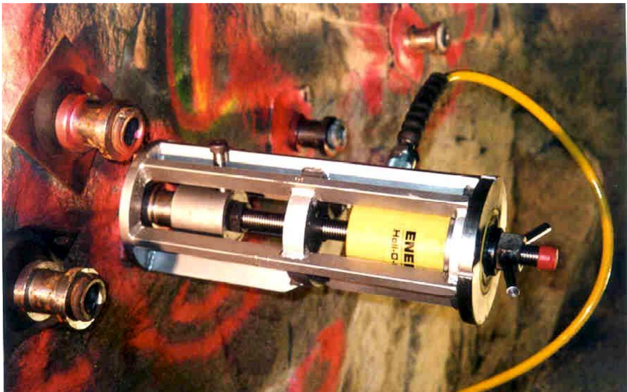
Fig. 6.5: Anchor pull-out test in the field
