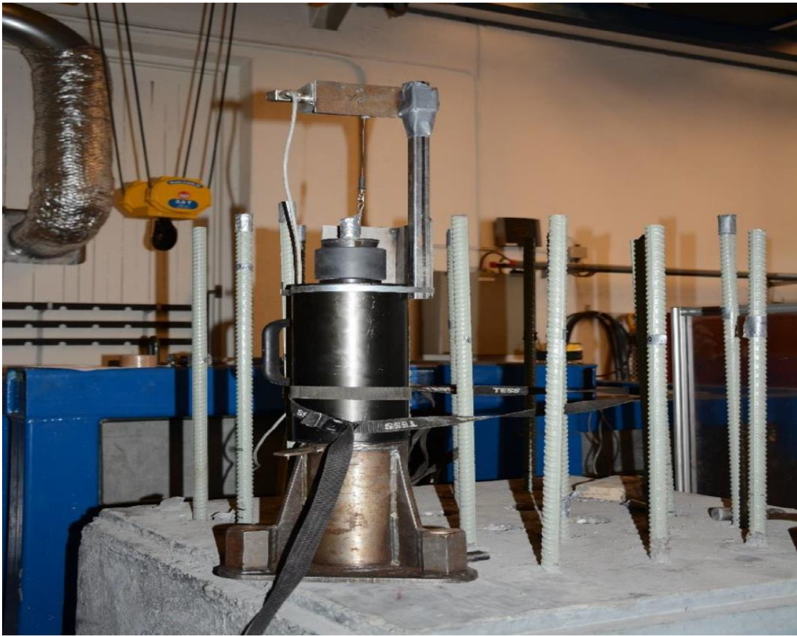
Fig. 6.2: Lab test set-up for pull-out-test (Kristjansson 2014)
