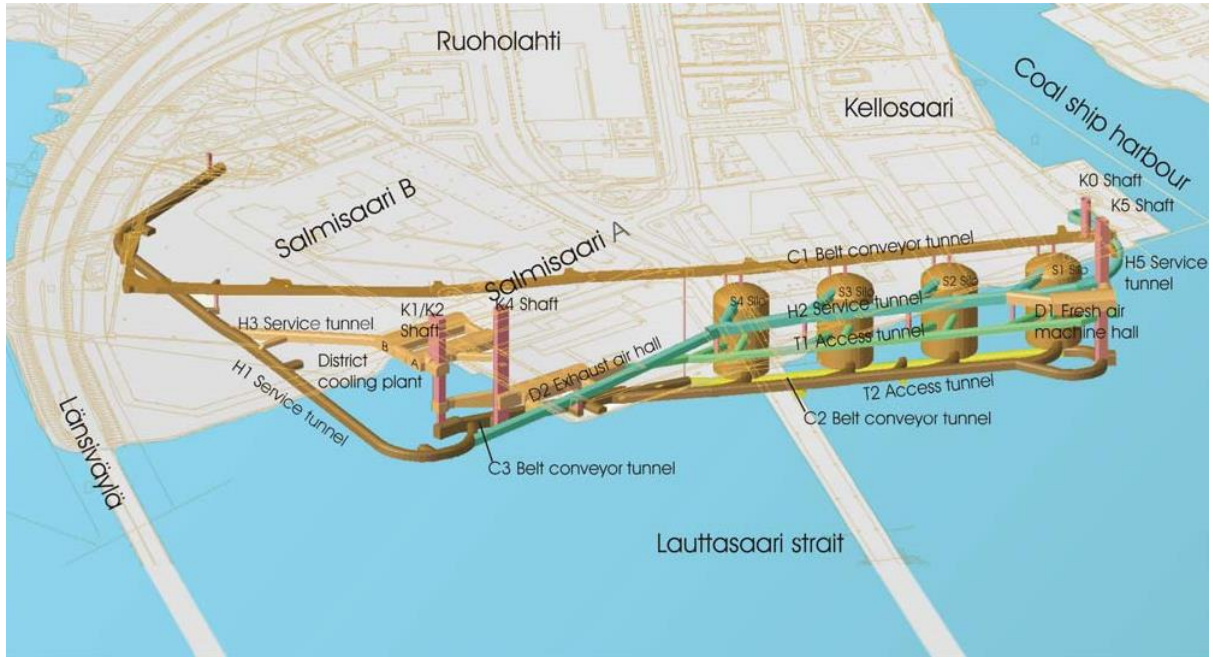
Fig. 7.4: Underground coal storage (Rockplan, 2020)
