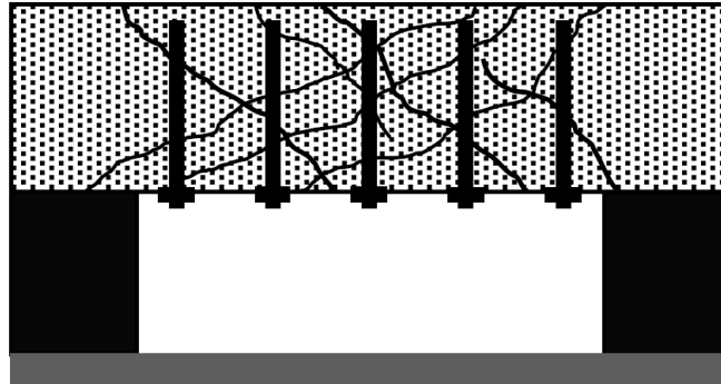
Fig. 2.3: Wedging effect mechanism
