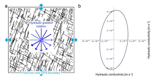
Fig. 9. (a) DFN with an edge length of 25 m. The dark-blue arrows indicate the rotation of the hydraulic gradient in steps of 30° until the gradients cover a total of 180°. The light-blue arrows indicate the fluid flux over the DFN boundaries. (b) The hydraulic conductivity tensor of the DFN shown in (a).
