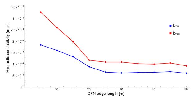
Fig. 10. Plot of DFN edge length against minimum ( $k_{min}$ ) and maximum ( $k_{max}$ ) hydraulic conductivity for quadratic fracture networks (chapter 5, Fig. 6b). The DFN have the same stochastic properties. All DFNs with an edge length of 25 m have a REV.
