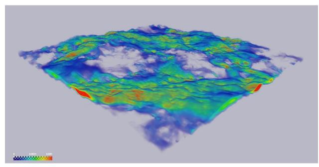
Fig. 8. Velocity field for the fluid transported through a rough fracture. Shown is the fracture void. The color code indicates the fluid velocity, with the highest velocities represented in red. Uncolored regions indicate areas where fracture surfaces touch, thereby forming rock bridges.
