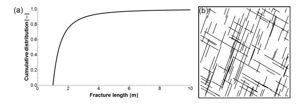
Fig. 6. (a) Plot of fracture lengths against their cumulative distribution for a truncated power-law function ( Eq. 12) with a lower cut-off  $l_0$  of 1m and an exponent  $E_{2D}$  of 2. (b) Ten by ten meter window of a 2D-DFN generated using the non-commercial software tool FracFrac (Blum et al., 2005). The fracture network consists of two sets with constant fracture strikes of 30° and 110° and fracture densities of 0.3 m<sup>-2</sup> and 0.7 m<sup>-2</sup>.
