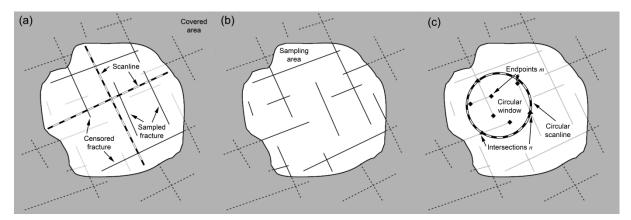
Fig. 5. (a) Scanline sampling, (b) window sampling, and (c) circular estimator method (modified from Rohrbaugh et al., 2002). Solid black lines indicate sampled fractures, light gray lines indicate non-sampled fractures and dashed lines non-observable (censored) parts of fractures (Zeeb et al., 2013).
