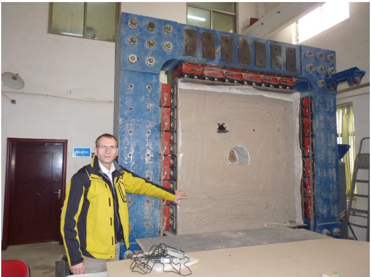
Fig. 9.1: Loading frame with physical model of tunnel with installed anchors (State key lab, Zhengzhou, China)
