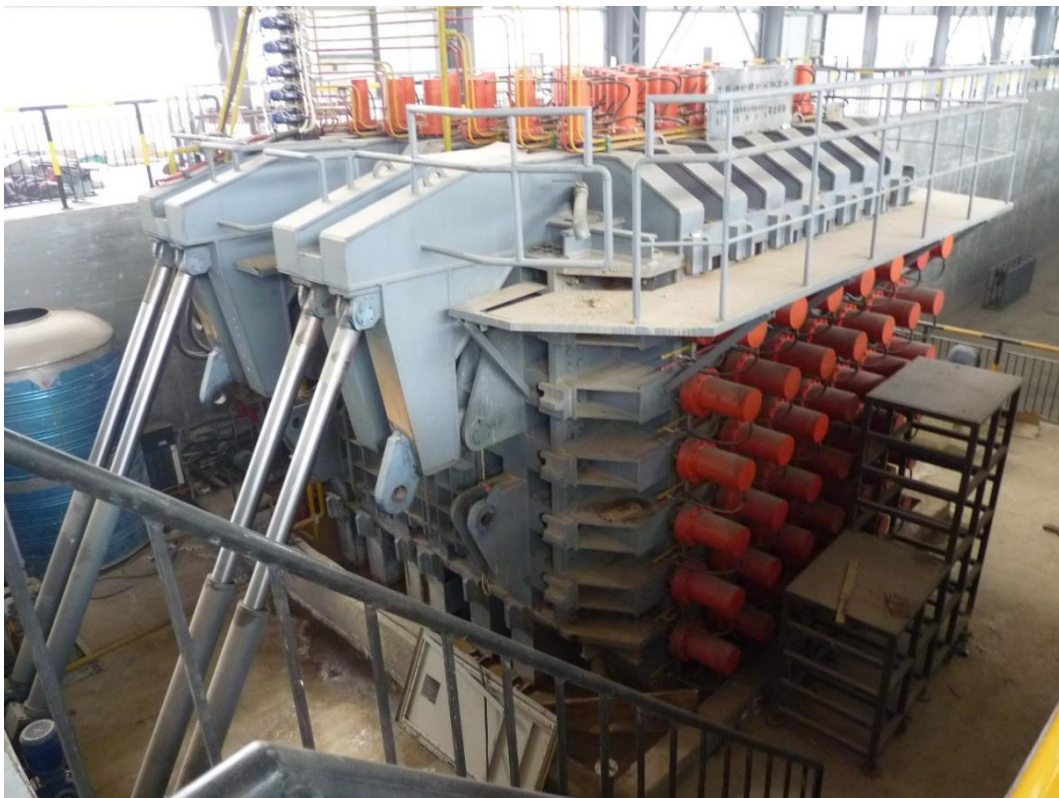
Fig. 9.3: True triaxial cell for large samples up to 3 x 3 x 3.5 m (State key lab, Zhengzhou, China)
