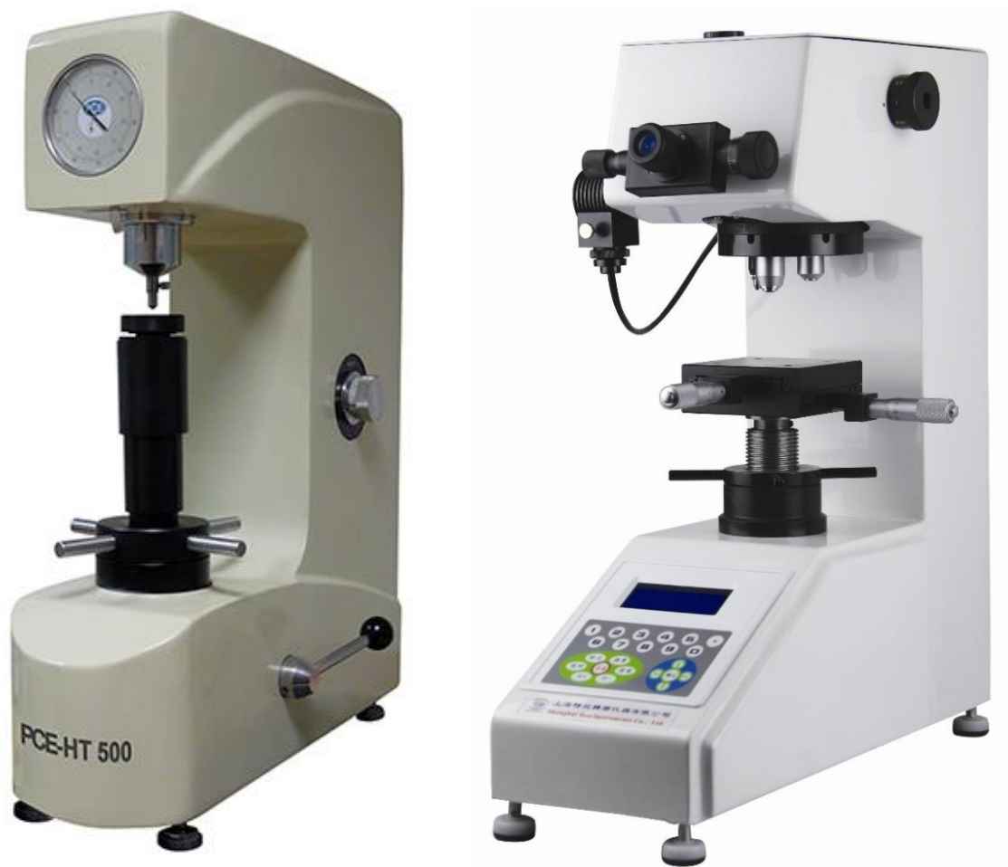
Fig. 3.1.4: Typical hardness testing devices [company leaflets]
