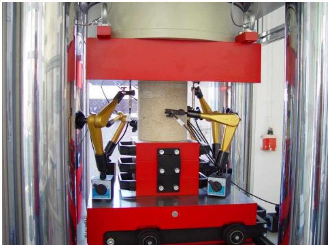
Fig. 3.7.2: Sample, prepared for uniaxial compression testing with longitudinal and lateral strain measurement direct on the sample [RML 2016]
