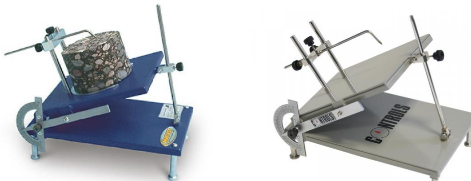
Fig. 3.11.2: Tilt test equipment (company material)
