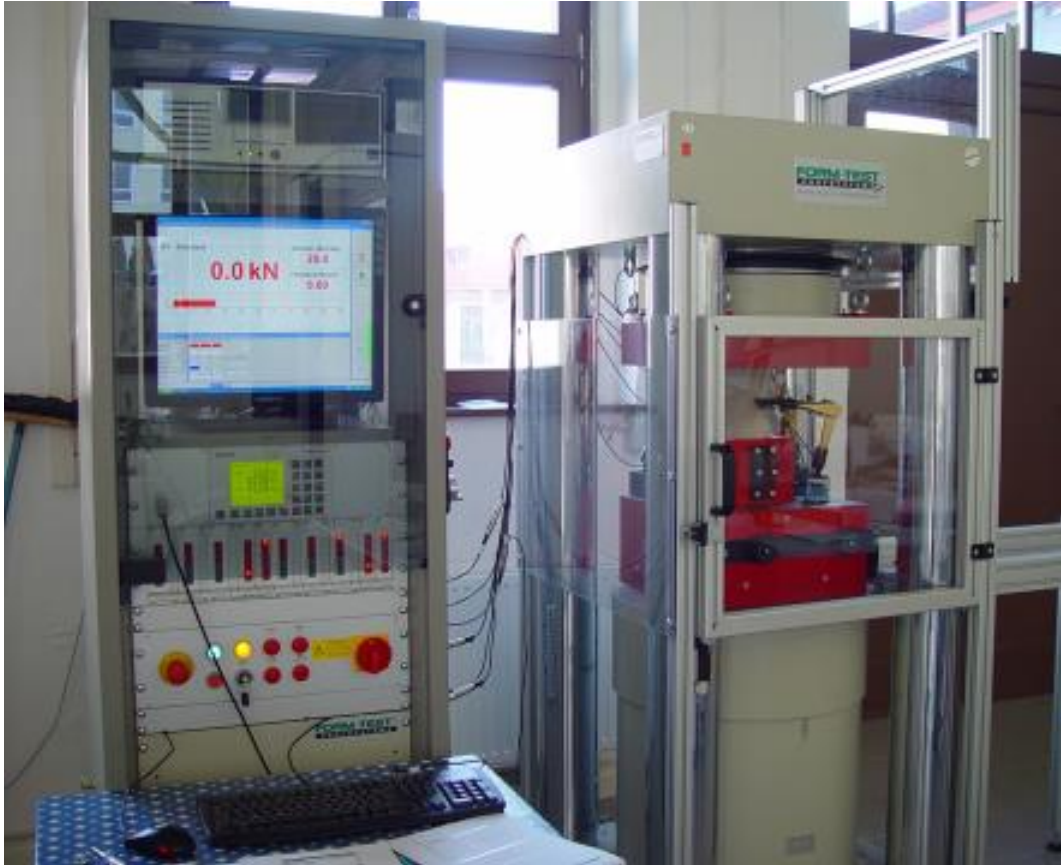
Fig. 3.7.1: Typical machine for uniaxial compression tests [RML 2016]
