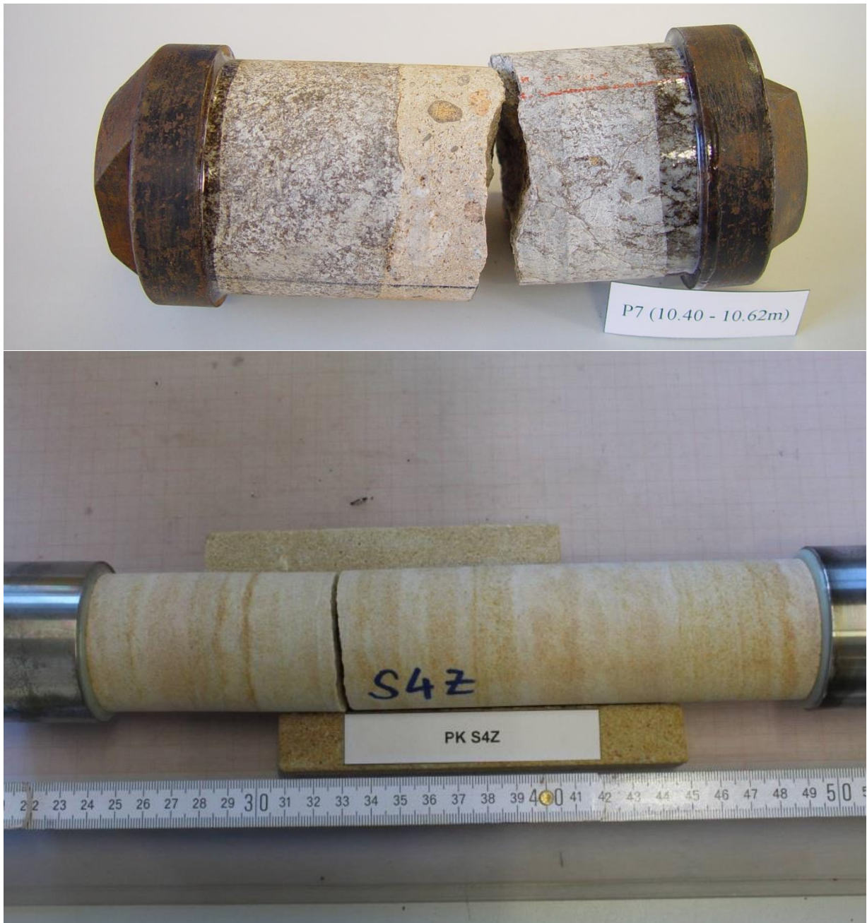
Fig. 3.8.2: Uniaxial tension test: Samples with typical failure pattern [RML 2016]
