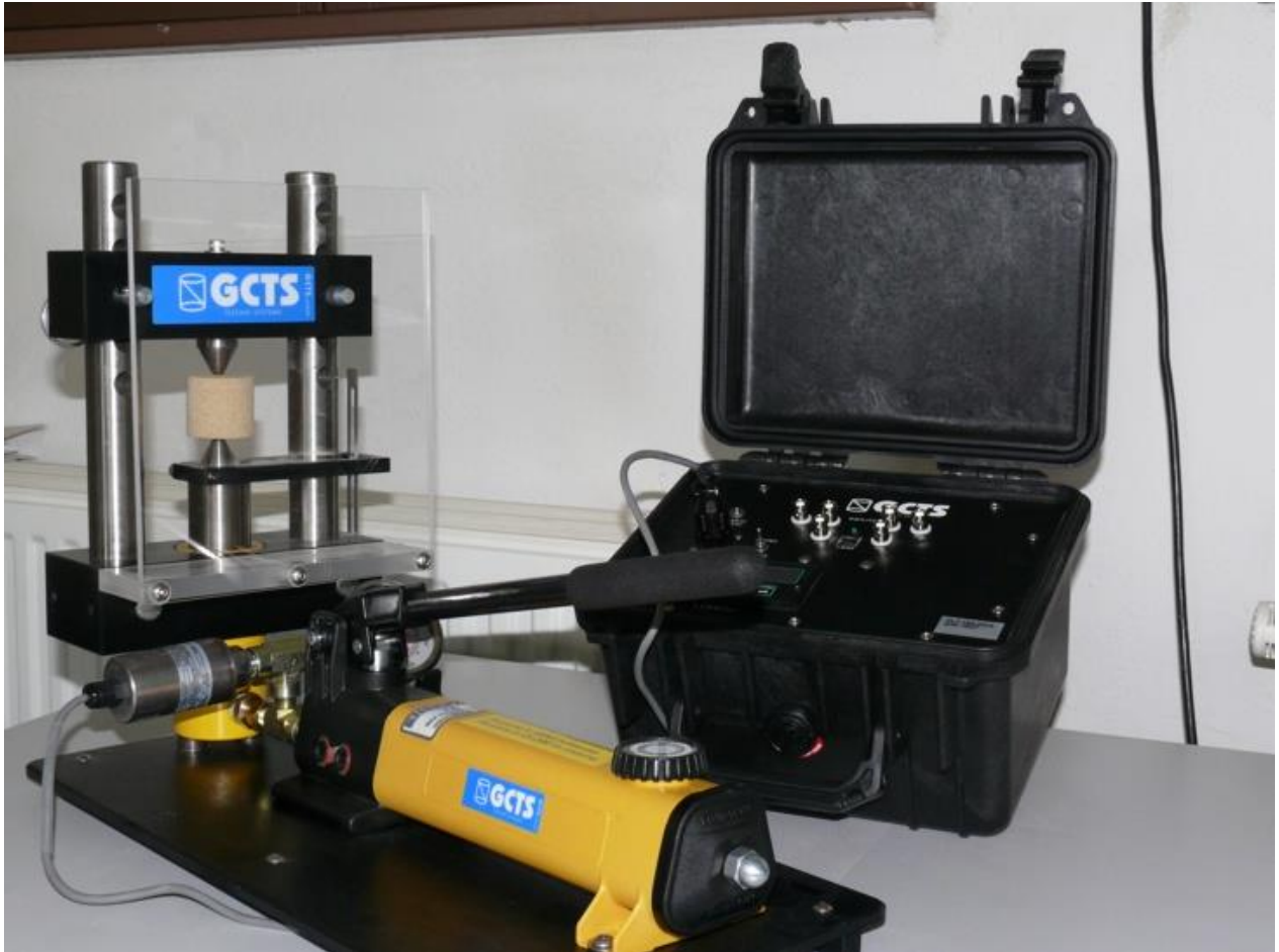
Fig. 3.4.1: Point Load Index Device (loading frame, pump with manometer and data acquisition unit) [RML 2016]
