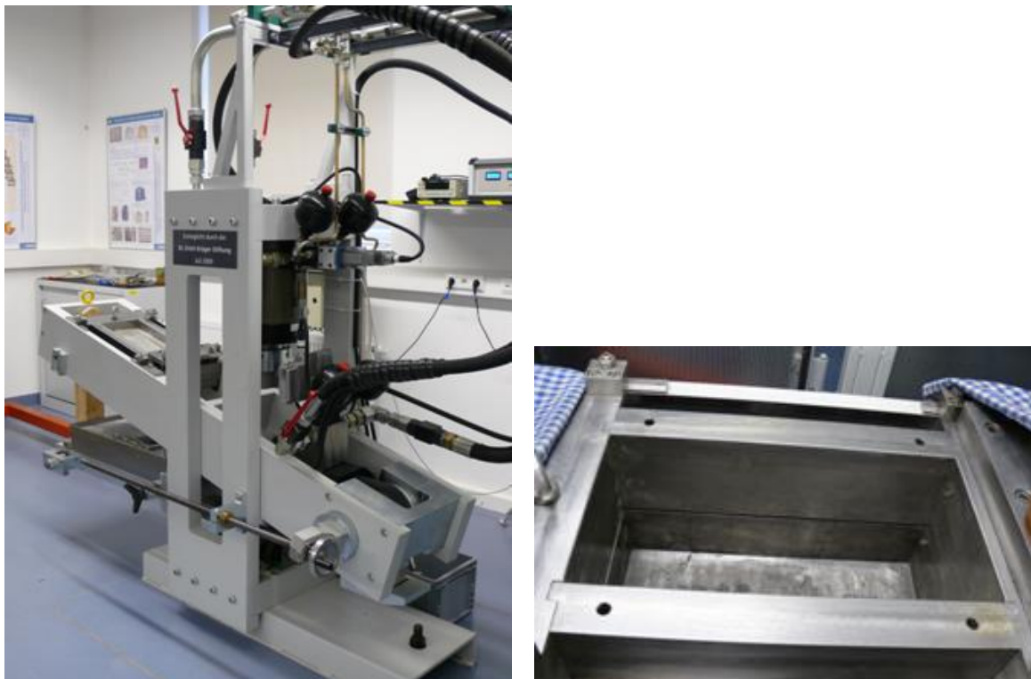
Fig. 3.14.2: Foto of a shear box device and view into empty shear boxes [Konietzky et al. 2012]
