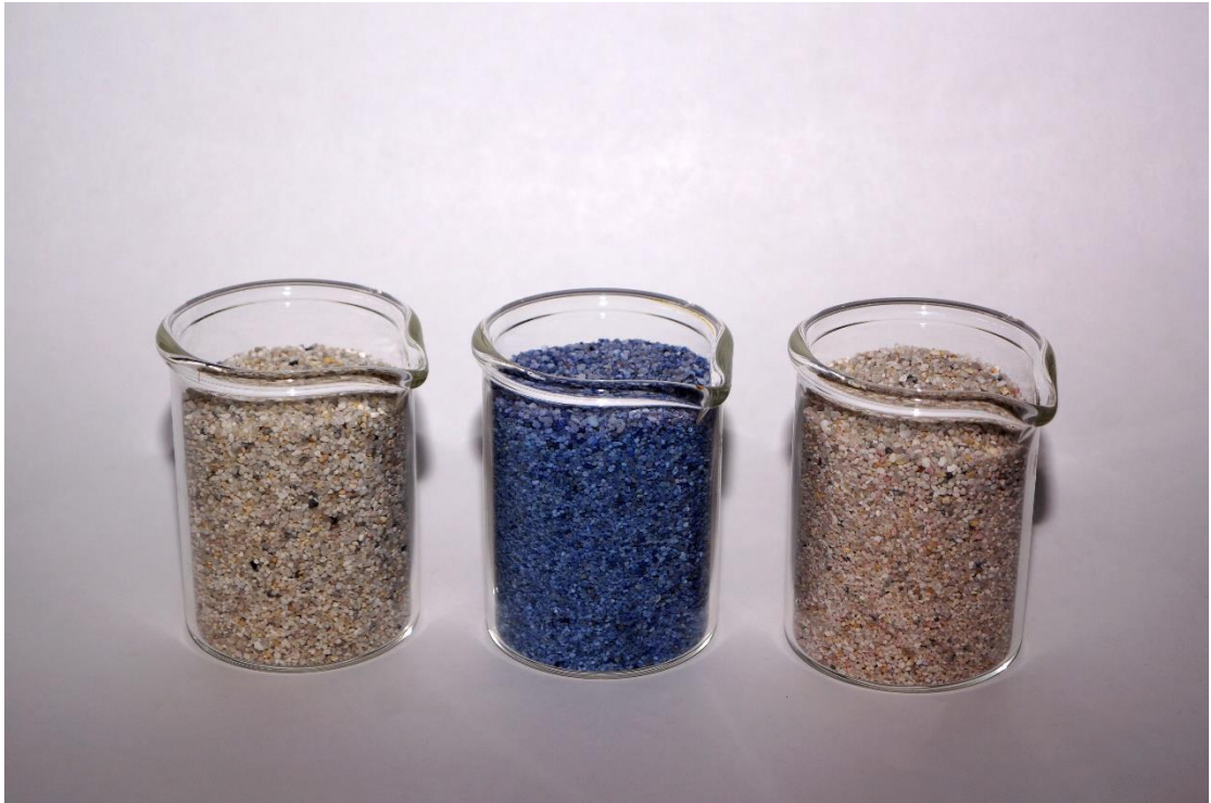
Figure 4. 1 Photograph of sand materials from three columns flushed with Orange II, methylene blue and reactive red 120 respectively. Pictures are from the work of Phukan 2015.
