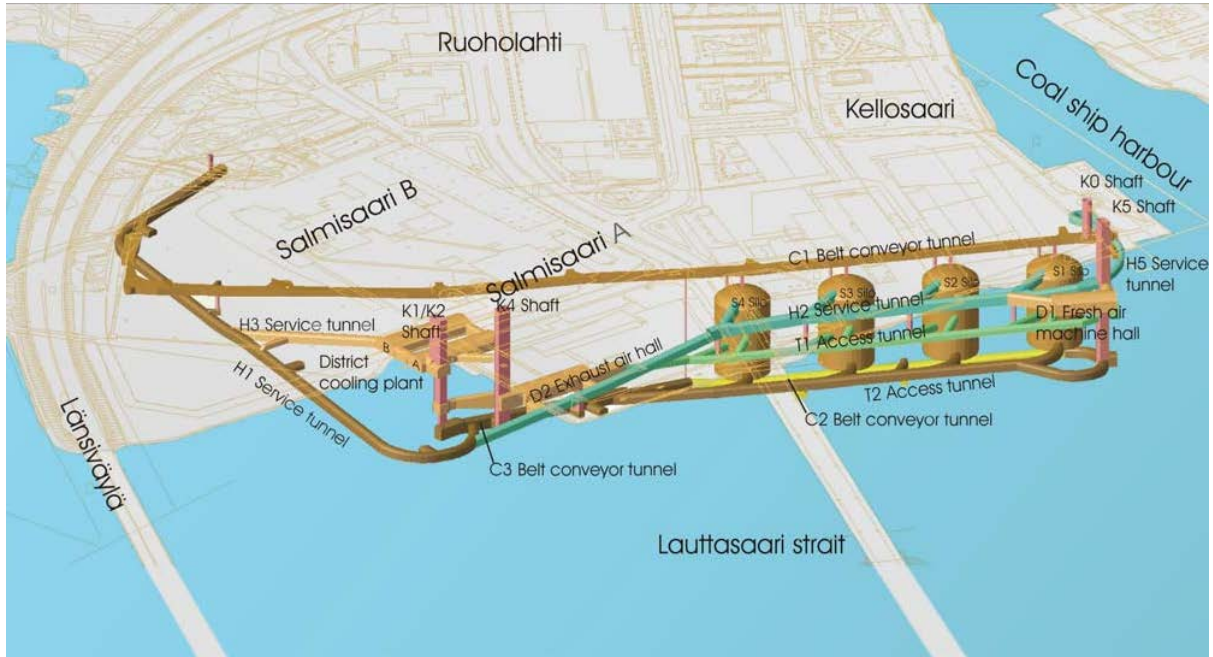
Fig. 7.4: Underground coal storage (Rockplan, 2020)
