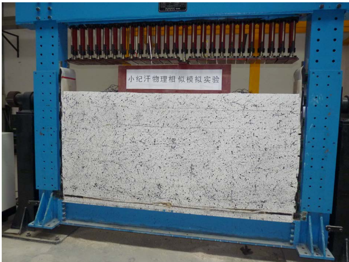
Fig. 3.1: Physical model prepared for image correlation via sprayed surface (China)
