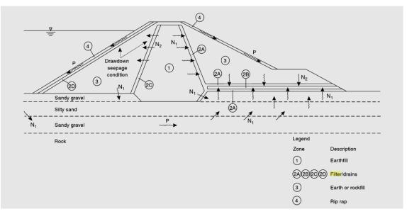
Fig. 4.1: Filters and flow conditions (P: flow parallel to interface, N<sub>1</sub>: Flow with high gradient normal to interface, N<sub>2</sub>:Flow with low gradient normal to interface) (Fell et al., 2015)
