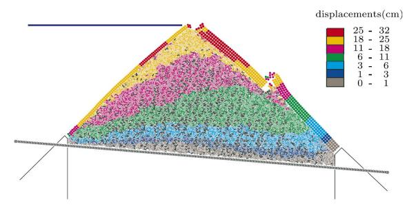
Fig. 5.4: Exemplary: 2D numerical model to simulate failure of rockfill dam using particle based Discrete Element Method (Deluzarche & Cambou,2006)
