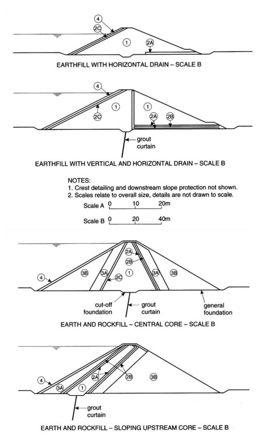
Fig. 4.2 (II): Typical embankment dam structures (Fell et al., 2015)
