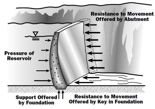
Fig. 3.3: Simplified sketch to illustrate the force situation for an arch dam (TCEQ, 2011)
