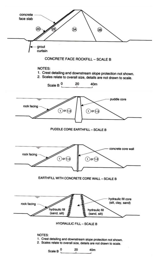
Fig. 4.2 (III): Typical embankment dam structures (Fell et al., 2015)
