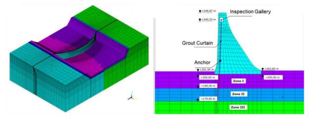
Fig. 5.3: Exemplary 3D numerical dam model (Schlegel et al., 2017)
