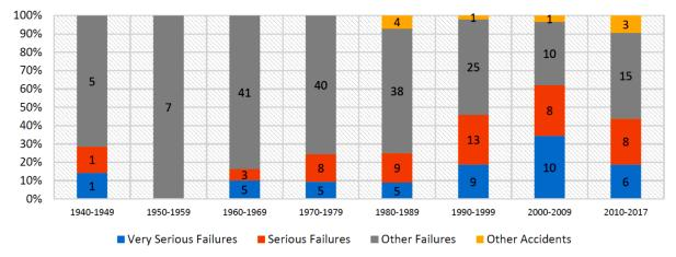
Fig. 8.2: Time-line and severity of global reported tailing dam failures (STINGS, 2018)
