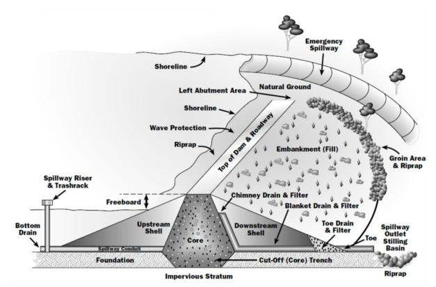
Fig. 1.4: Dams: basic construction and technical terms (TCEQ, 2011)
