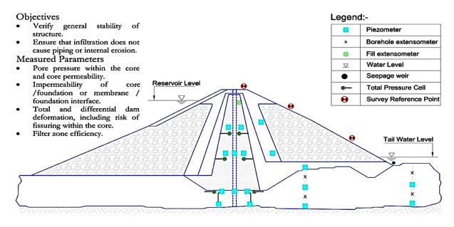
Fig. 7.4: Illustration of a typical monitoring system for an embankment dam (CWC, 2018)
