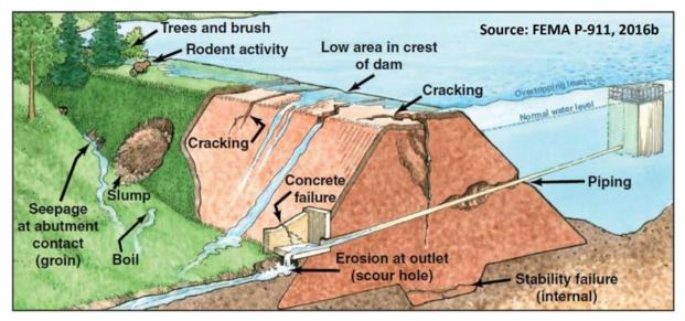
Fig. 8.1: Illustration of typical modes of water dam failures (CRS, 2019)
