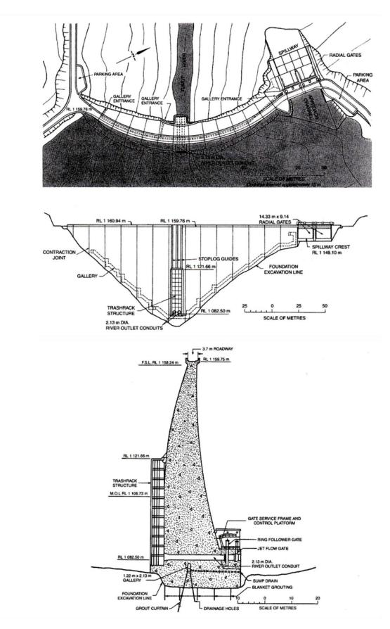
Fig. 3.4: Typical arch dam plan (Fell et al., 2015)
