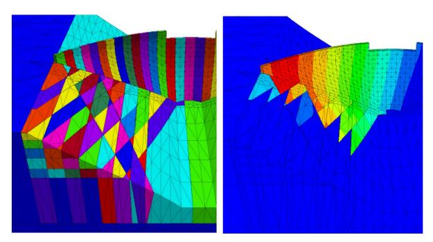
Fig. 5.3: Exemplary: 3D numerical dam model with explicit consideration of rock joint pattern using Discrete Element Method (Lemos, 2012)
