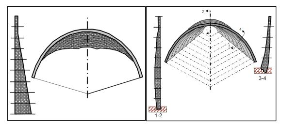
Fig. 3.2: Sketch illustrating different types of arch dams (Yurtal, 2020)
