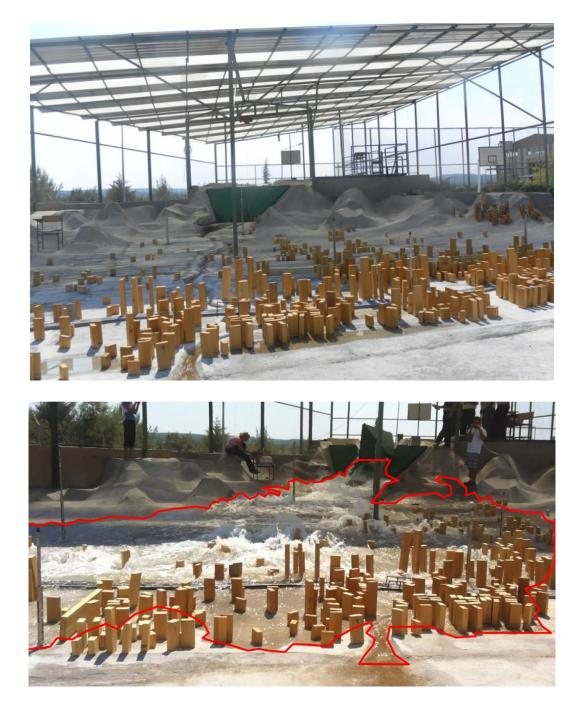
**Fig. 5.5:** Physical model to simulate dam breakage and flooding (Güney et al., 2014)
