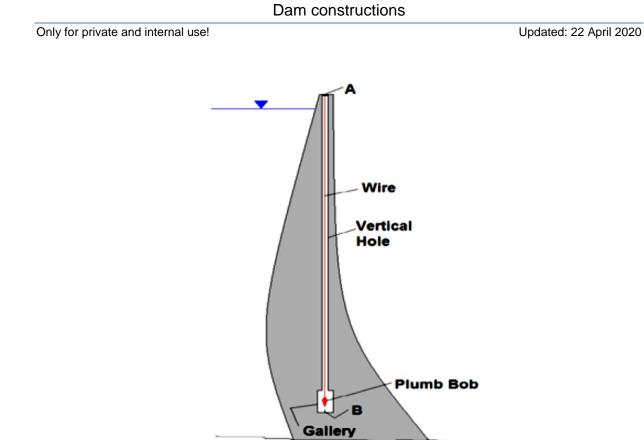
Fig. 7.2: Plumbline installed in an arch dam (FERC, 2018)
