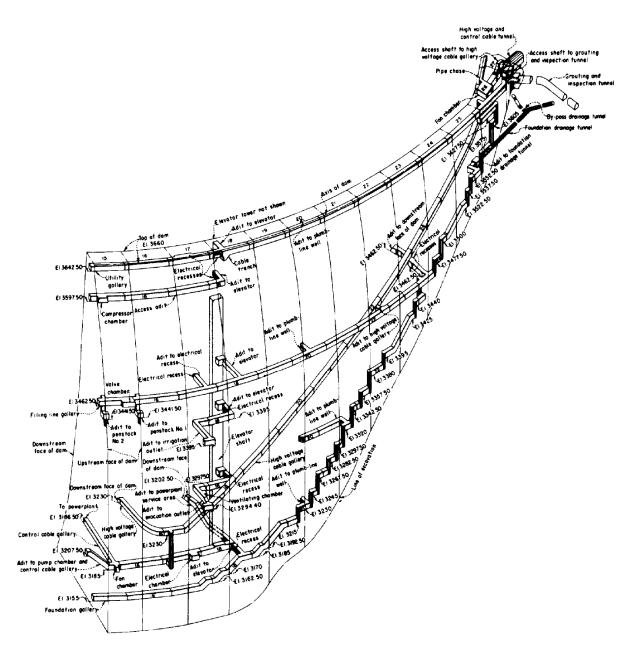
Fig. 3.5: Right abutment of Yellowtail arch dam (ACE, 1994)
