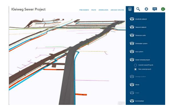
Fig. 5.3.2: BIM model for Kleinweg Sewer Project with streets and underground network layers only (Nie, 2019)
