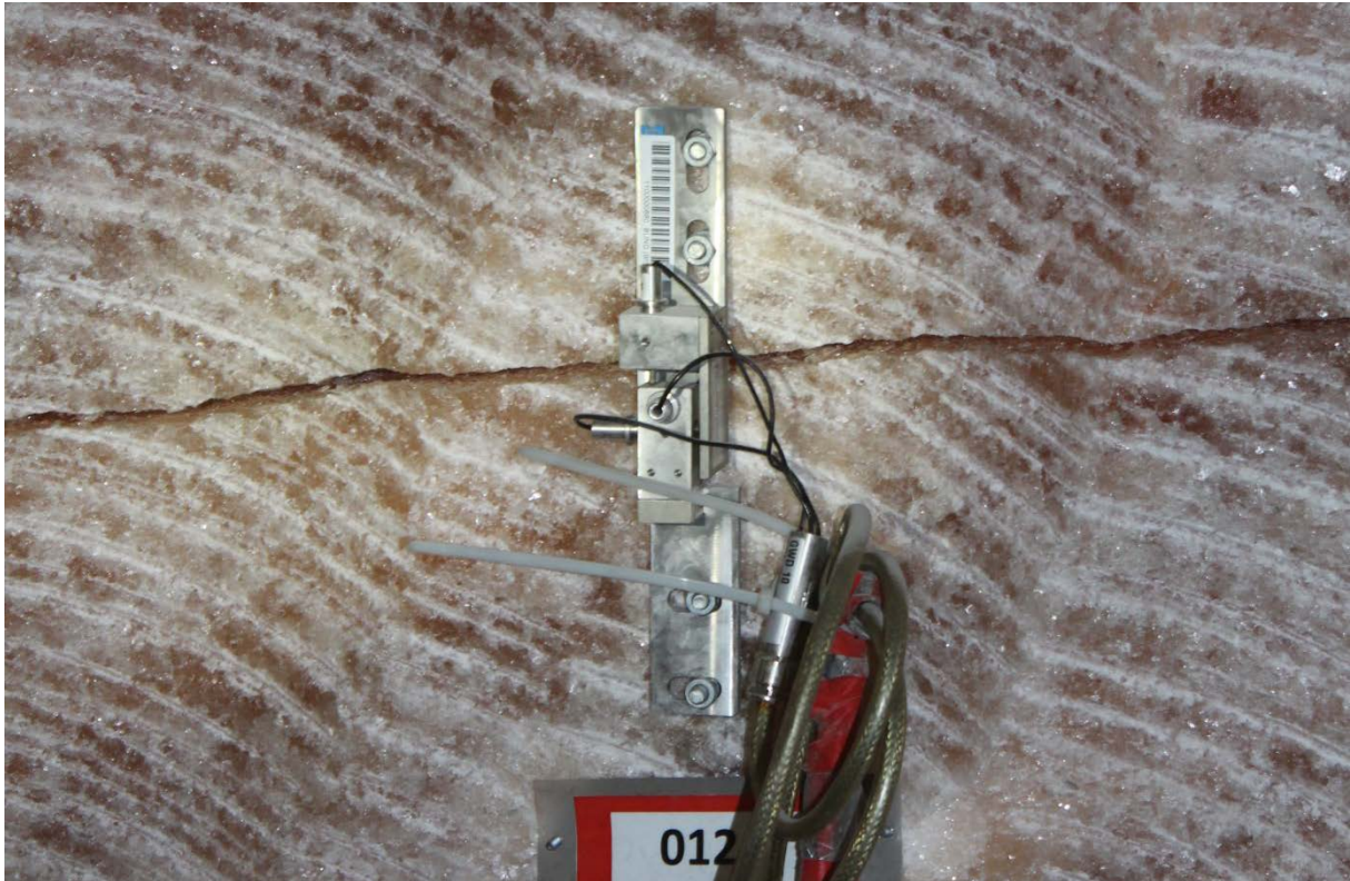
Fig. 4.8.4: Crackmeter (installation in an underground mine)
