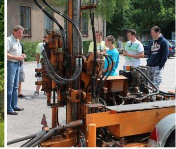
Fig. 19: Mobile trailer drill rig (RML 2016)
