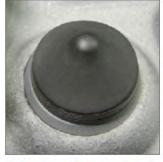
WT-No wear (Level 0 severity)
