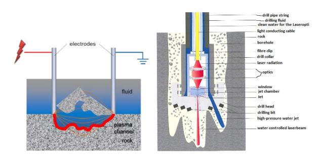
Fig. 30: Scheme of EIT (left) and laser drilling (right) (Richter, 2017)
