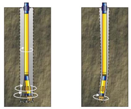
Fig. 2. Principle of rotary steerable systems (company material)
