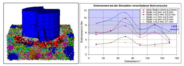
Fig. 28: Simulation of drilling process and comparison with moments measured in the lab (Lunow 2015)
