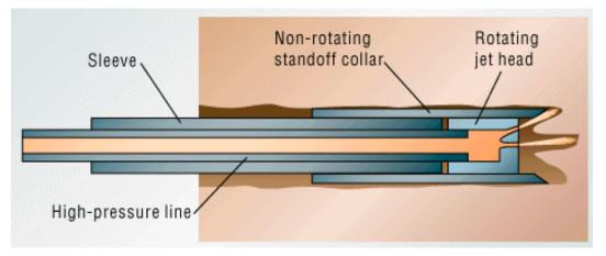
Fig. 6: Water jet drilling (company material)
