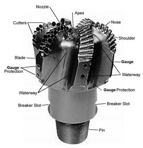
Fig. 14. Principle design of PDC drill bits (company material)
