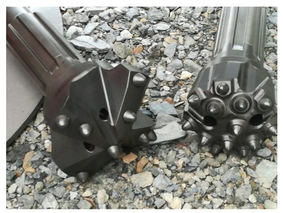
Fig. 15: Drill bits for small scale holes
