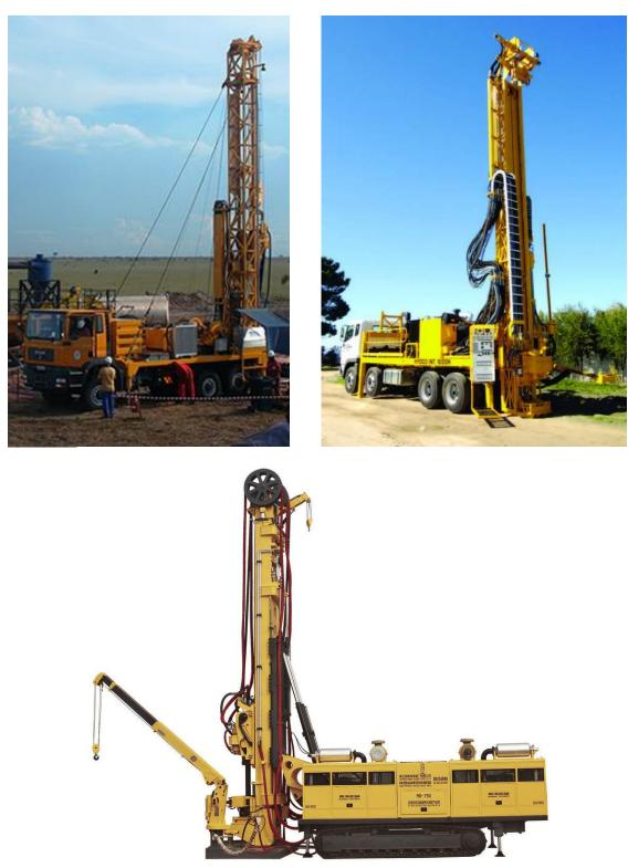
Fig. 18: Mobile self-driven drill rigs (company material)
