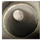
WT – Minor wear (Level 2 severity)
