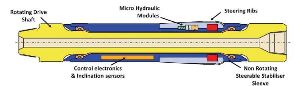
Fig. 4: Sketch of steering mechanism (company material)
