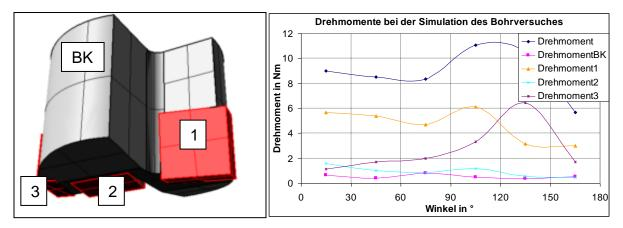
Fig. 29: Drilling head with three inserts and simulated moments acting on these parts (Lunow 2015)
