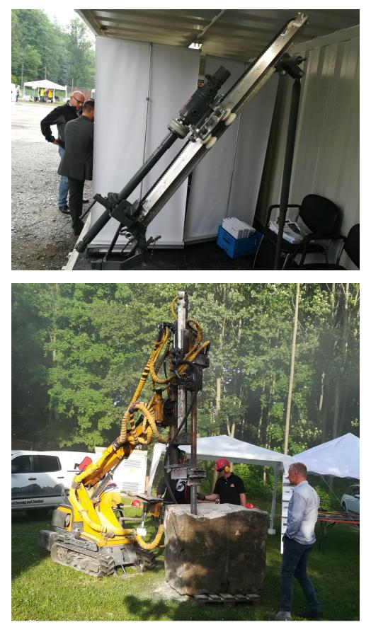
Fig. 17: Portable drill rigs for small scale holes
