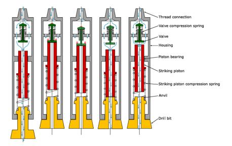
Fig. 31: Scheme of hydraulic downhole hammer (Richter, 2017)
