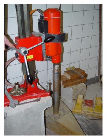
Fig. 24: Lab drill rig to extract cores from rock blocks (RML 2017)
