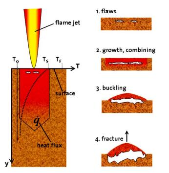
Fig. 8. Principal of hydrothermal spalling drilling (www.transfer.ETH.ch)
