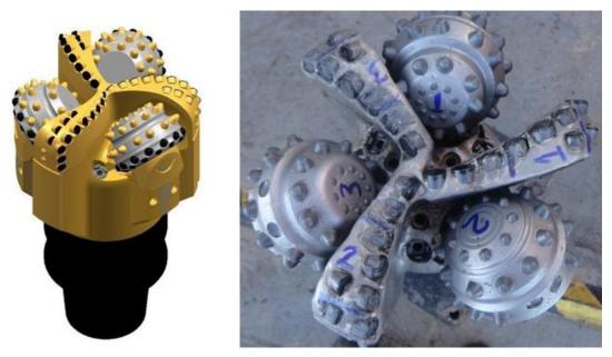
Fig. 11: Hybrid drill bit with PDC cutters for large holes and deep drilling (company material)
