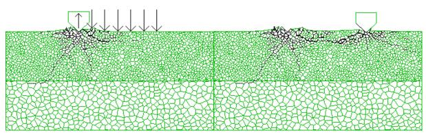
Fig. 27: Simulation of rock fragmentation due to penetration of a single disk cutter (Lunow & Konietzky 2010)
