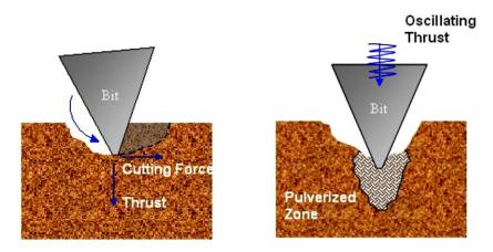
Fig. 26: Principal of rock fragmentation in rotary (left) and percussion (right) drilling (Terralog 2005)
