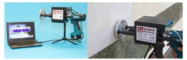
Fig. 23: Drilling resistance measuring device (company material)
