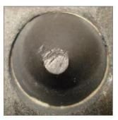
WT – Minimal wear (Level 1 severity)
