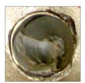
DL-Stinger element delamination
