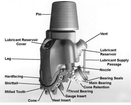
Fig. 13. Principle design of roller cone bits (company material)
