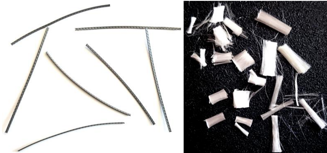
Fig. 12: Synthetic macro-fibers (left) and micro-fibers (right), (company material from Sika).
