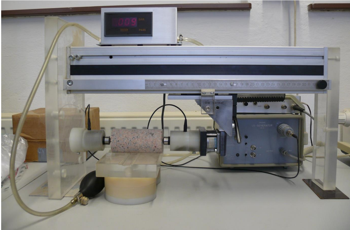
Fig. 3.6.1: Typical equipment to measure sound velocity on core samples [RML 2016]
