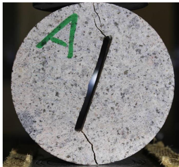
Fig. 3.15.3: Test set-up for CCNBD test [RML 2016]
