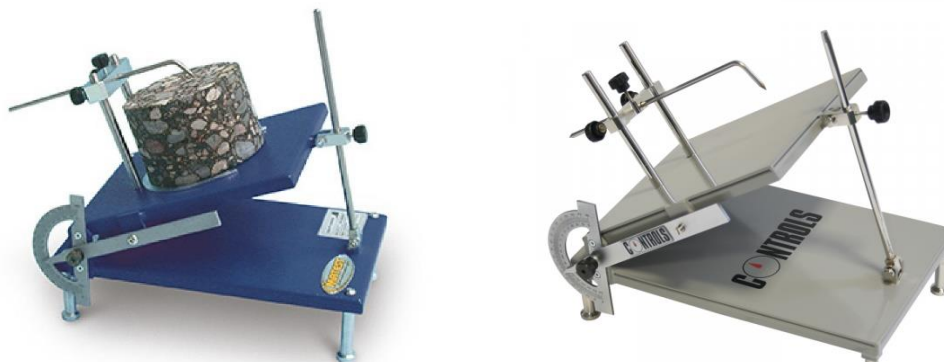
Fig. 3.11.2: Tilt test equipment (company material)
