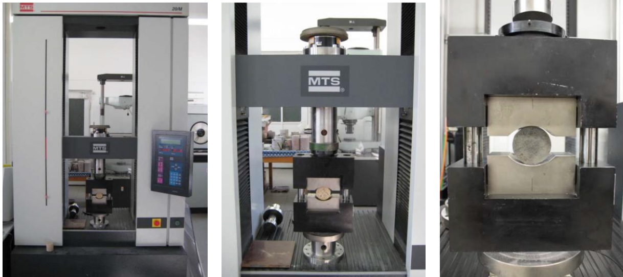
Fig. 3.9.3: Typical test arrangement with arc-formed loading jaws and cylindrical samples [RML 2016]
