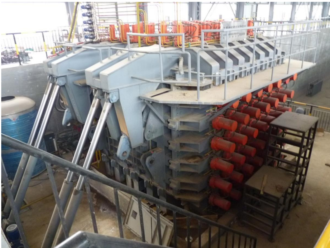
Fig. 7.3: True triaxial cell for large samples up to 3 x 3 x 3.5 m (State key lab, Zhengzhou, China)
