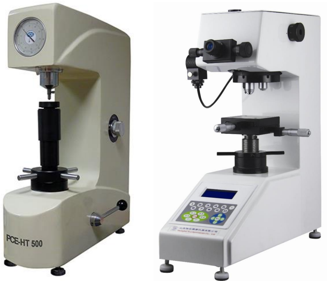
Fig. 3.1.4: Typical hardness testing devices [company leaflets]
