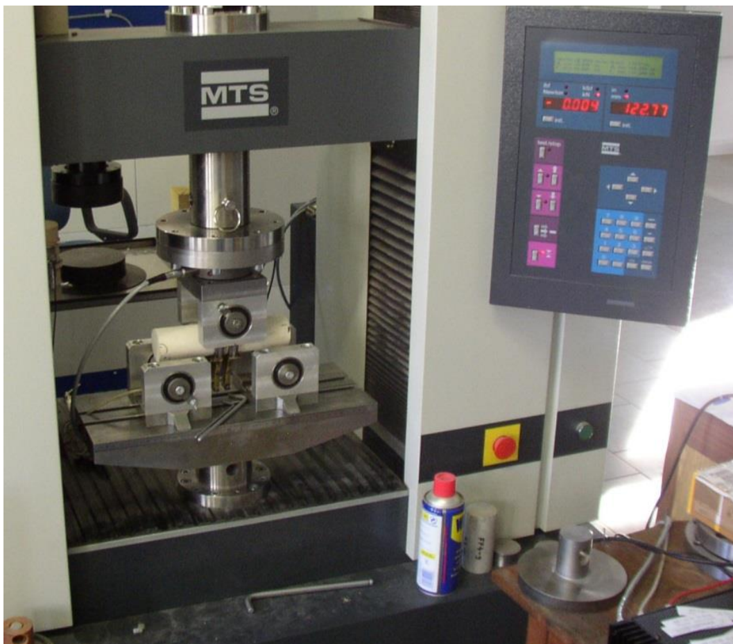
Fig. 3.15.1: Test set-up for CBS test [RML 2016]
