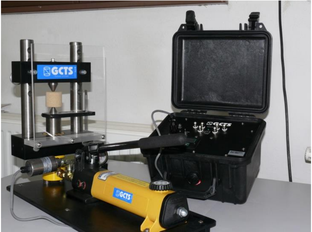
Fig. 3.4.1: Point Load Index Device (loading frame, pump with manometer and data aquisition unit) [RML 2016]
