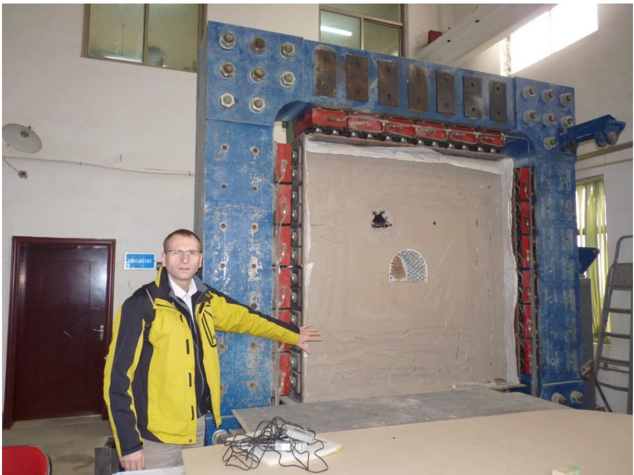
Fig. 7.1: Loading frame with physical model of tunnel with installed anchors (State key lab, Zhengzhou, China)
