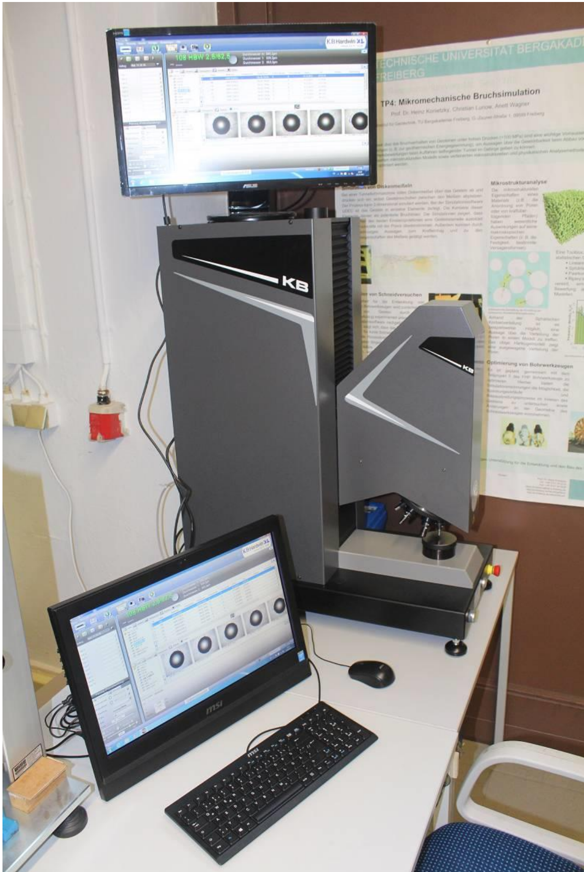
Fig. 3.1.5: Multi-functional hardness testing device with digital image analysis [RML 2016]
