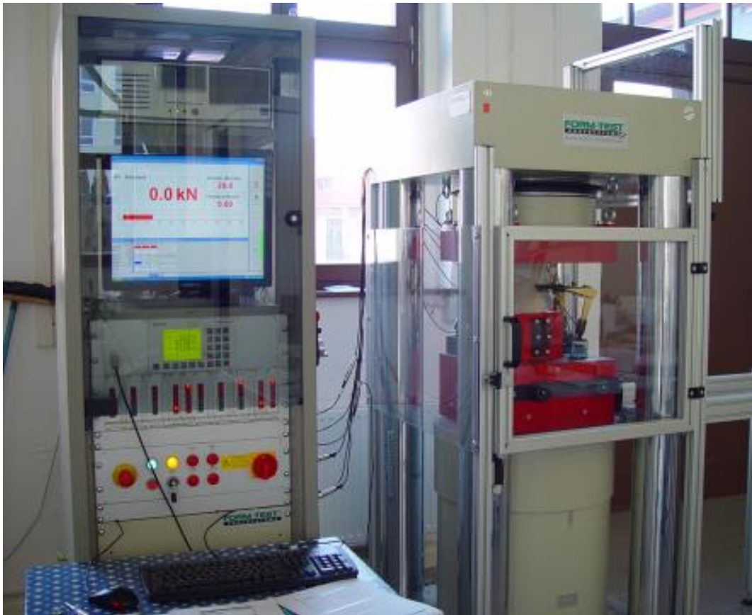
Fig. 3.7.1: Typical machine for uniaxial compression tests [RML 2016]
