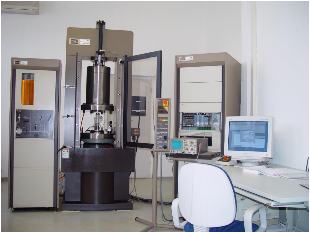
Fig. 3.12.2: Typical triaxial testing device with loading frame and triaxial cell, pressure unit and data recording unit [RML 2016]
