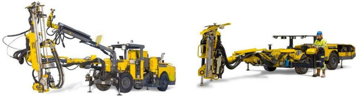
Fig. 7.1: Rock bolting rigs (Atlas Copco, company material)
