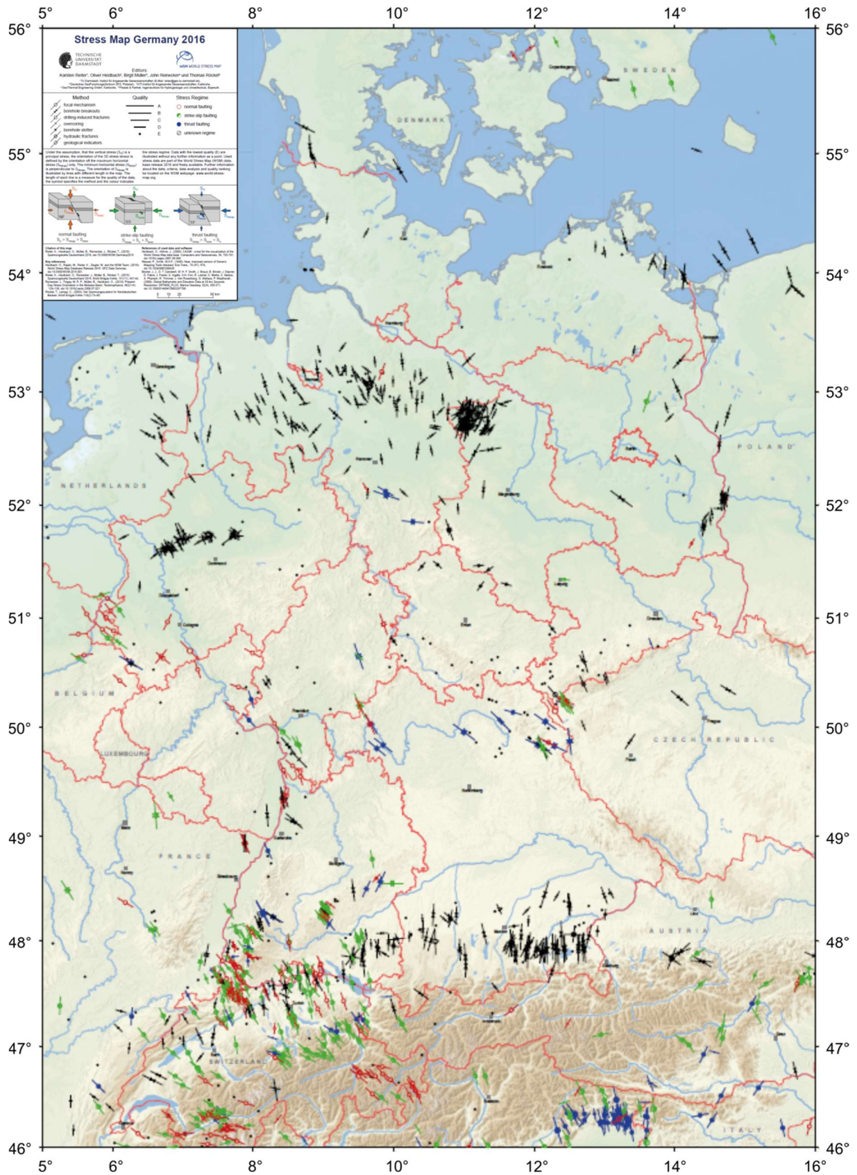
Fig. 2.4: Maximum principal stress orientation and stress regimes for Germany (modified after Reiter et al., 2016)
