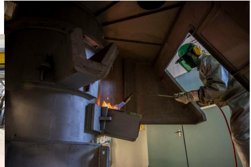
L. Blenau: Pilot Scale Top Submerged Lance (TSL) Furnace tap (top) and off-gas cleaning unit (left)
