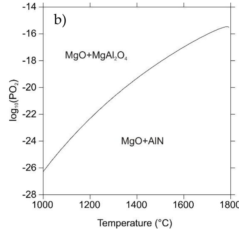
Equilibrium of MgAl<sub>2</sub>O<sub>4</sub> with MgO and AlN in presence of gas as a function of temperature: (a) activities of gas species; (b) partial pressure of oxygen.
