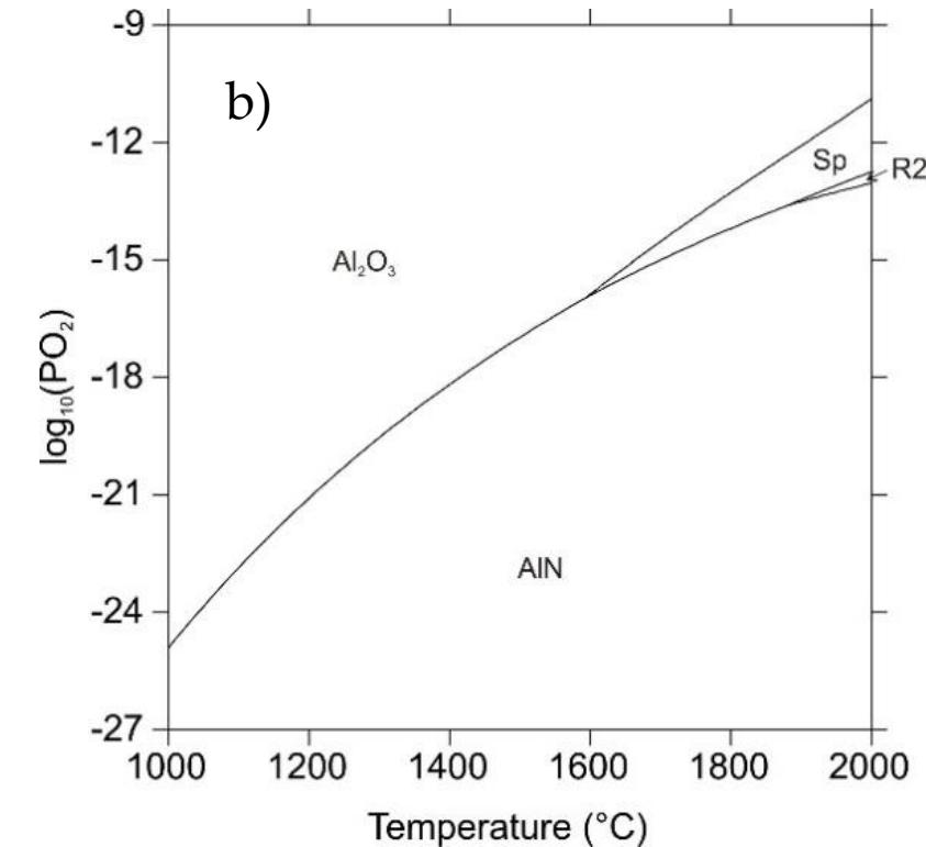
Phase equilibria in the  $\text{Al}_2\text{O}_3$ -AlN system  $\text{Al}_2\text{O}_3 + \text{AlN}$ ,  $\text{Al}_2\text{O}_3 + \text{Spinel AlON}$ , Spinel AlON+AlN, R27+Spinel AlON and R27+AlN in presence of gas: (a) temperature dependence of the activities of gas species; (b) temperature dependence of the partial pressure of oxygen.
