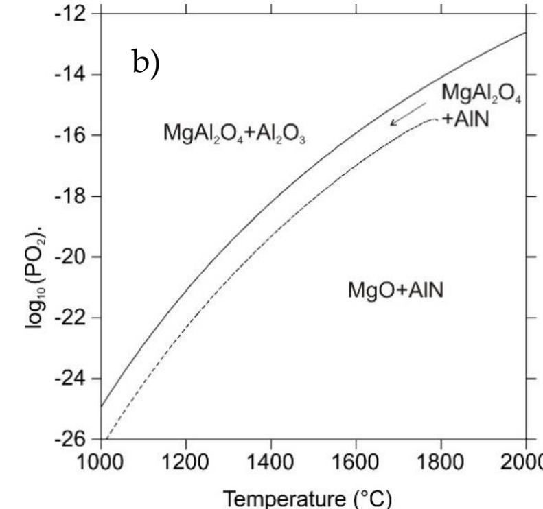
Equilibrium of  $\text{MgAl}_2\text{O}_4$  with  $\text{Al}_2\text{O}_3$  and  $\text{AlN}$  in presence of gas as a function of temperature:
