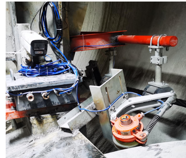
On-line non-destructive testing (NDT) of wire ropes
