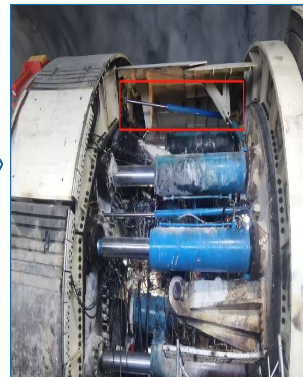
Horizontal-inclined cross stroke measuring cylinder
