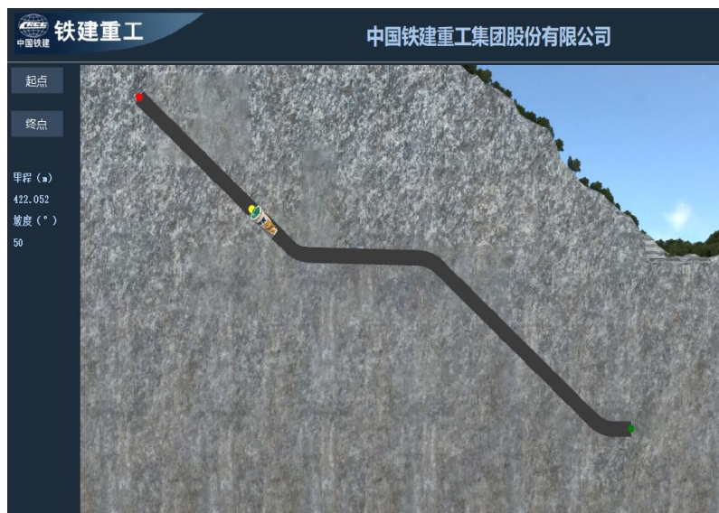
Active deviation correction control system for inclined shaft TBM
