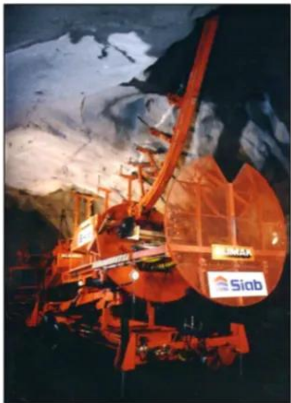
Alimak climber in protective position
