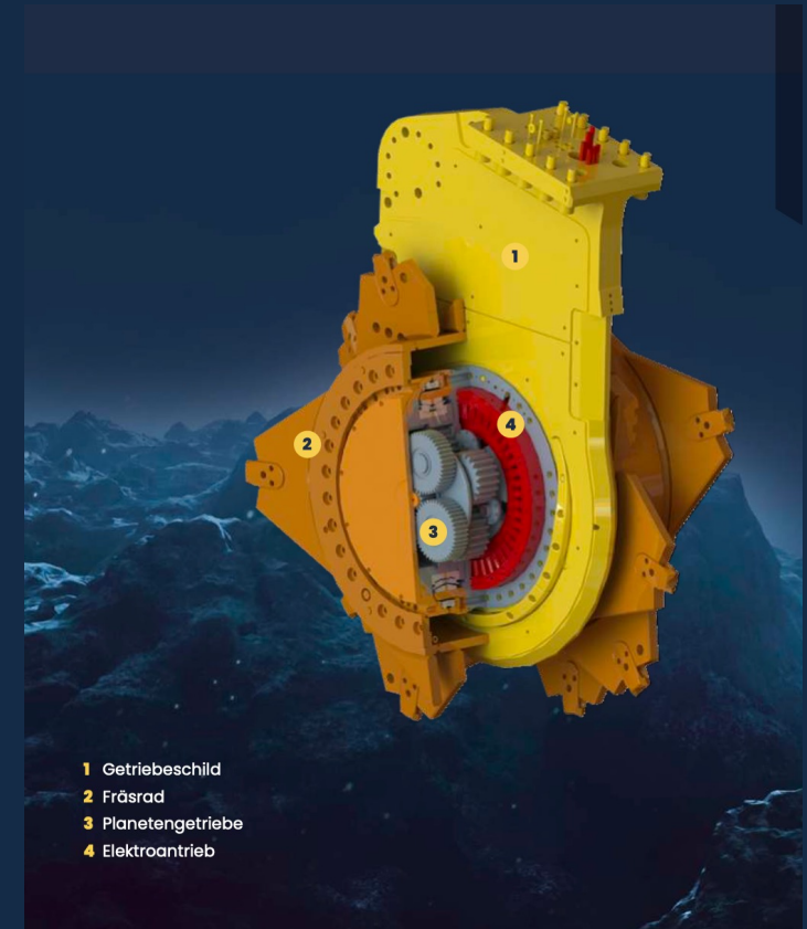
Sectional representation of the E-CSM
