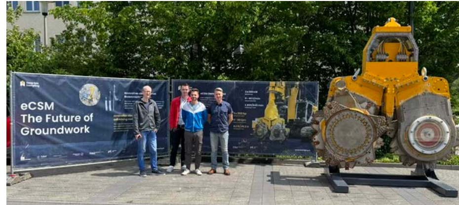
Freiberg, Summer 2025: fully electrified direct-drive cutter head after testing
