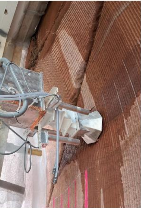
Irradiation of hard rock with high power microwaves
