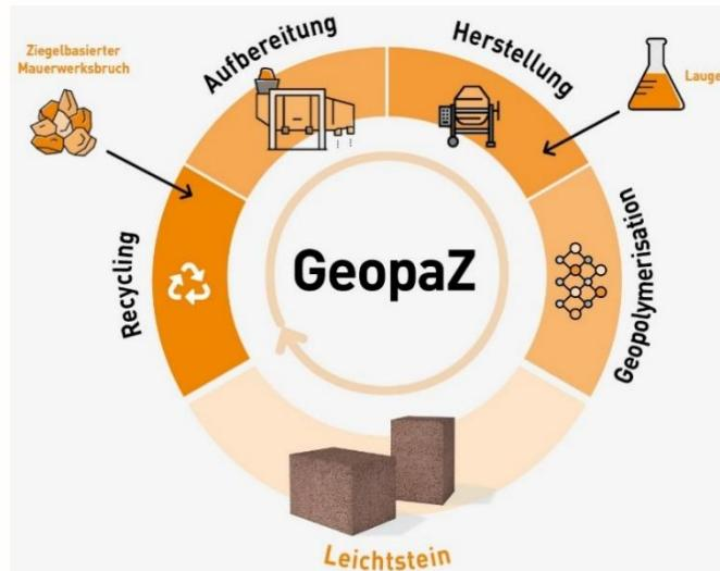
Production is carried out by mixing a three-component blend consisting of brick-based residual materials, an aqueous alkaline solution, and a secondary-raw-material-based foaming agent. The chemo-thermal activation takes place at temperatures between 60 and 100 °C.
