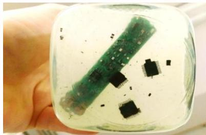
The *bio-dismantling* process detaches electronic components from circuit boards using a bacterial leaching solution. The bacteria
