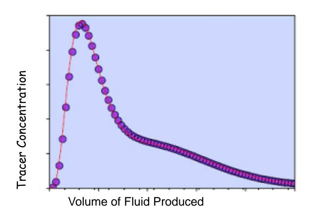
Breakthrough of Reinjected Water (Hydraulic Front) to Production Well
