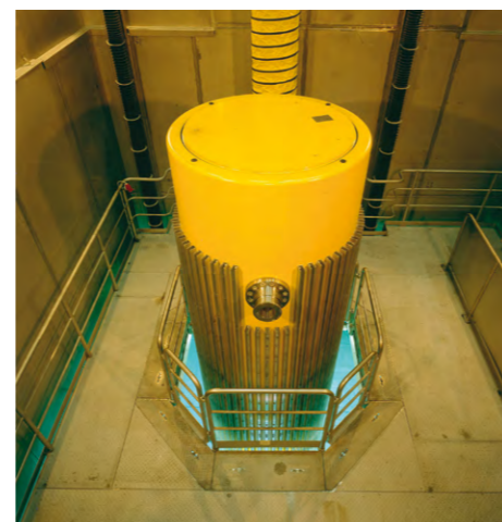
POLLUX® cask at a maintenance station of the Pilot Conditioning Plant at Gorleben (Germany)
