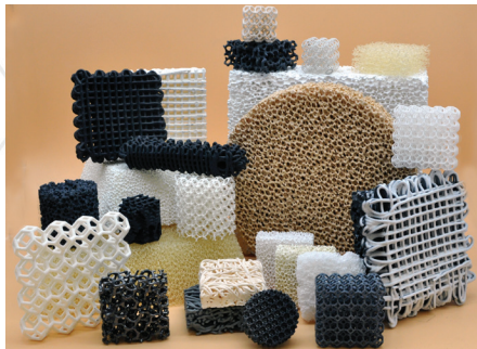
Photo: Filter components and structures for metal melt filtration, project area A.
