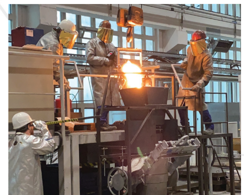
Photo: Impingement test at the Foundry Institute for suitability testing of newly developed metal melt filters.
