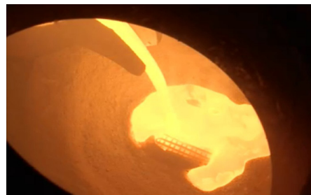
Photo: Test of filter structures in the cast steel simulator.
