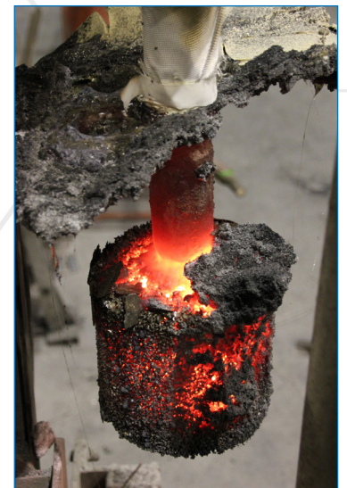
Fig. 2: Carbon-bonded alumina filter after application in industrial-scale continuous steel casting.
