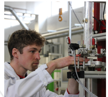
Photo: Fabian Heuzeroth inserts a filter, which was made in subproject A02, for experiments in the filtration testing stand.
