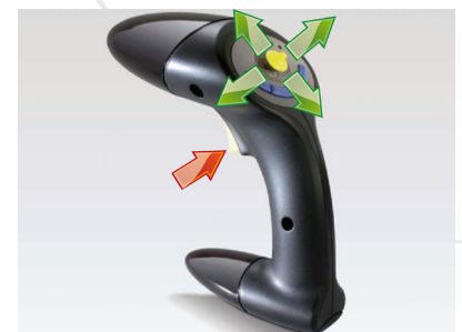
Fig. 3: The flystick provides tracking of position and orientation in 3D space and is used for navigation as well as seeding tracer particles/streamlines in the data set.
