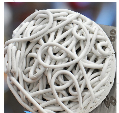
Figure: "Spaghetti" ceramic as basic structure for filter macro structures
